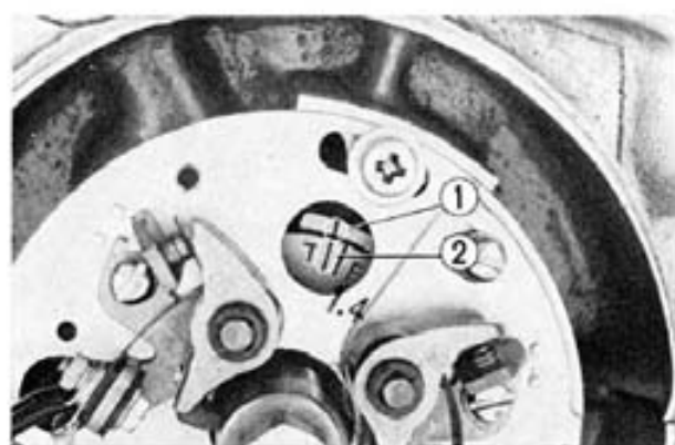
Fig. 3-56 ① Index mark ② "T" mark
