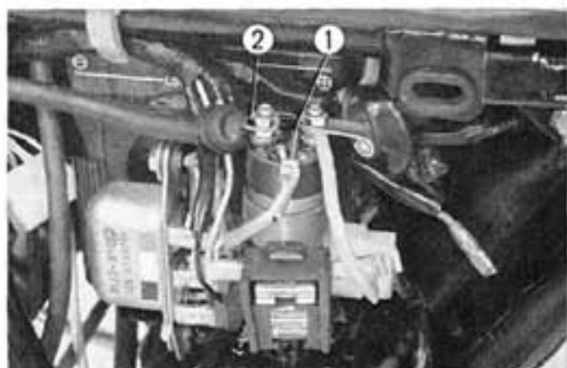
Fig. 9-3 ① Magnetic switch ② Starting motor cable
