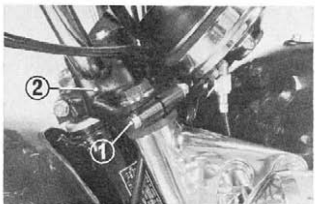
Fig. K6-6 ① 7mm flange bolt ② Fork top bridge
