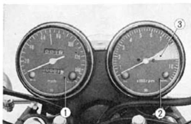
Fig. 20-34 ① Speedometer ② Tachometer ③ Red zone
