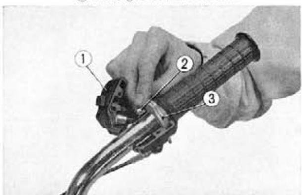
Fig. 16-17 ① Starter lighting ignition switch assembly ② Throttle cable ③ Throttle control
