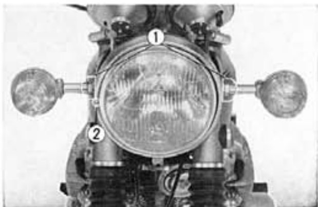
Fig. 19 21 ① Headlight mounting bolts ② Adjusting screw
