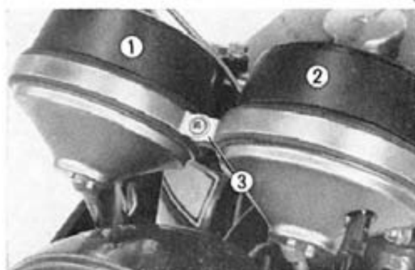
Fig. 16-2 ① Tachometer ② Speedometer ③ Setting screw
