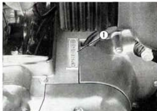
Fig. 1-2 ① Engine serial number
