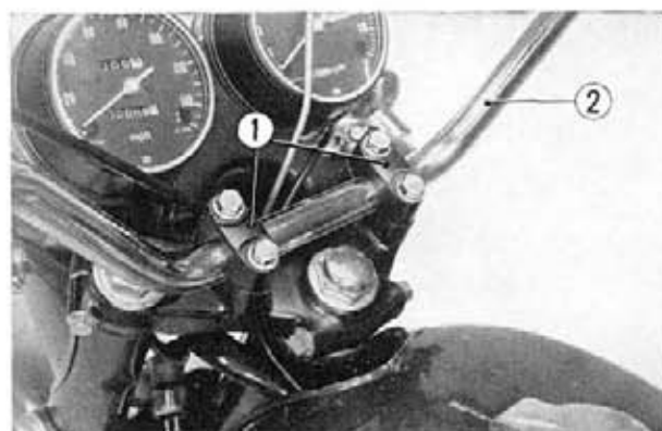
Fig. 11-3 ① Upper handle holders ② Handle bar
