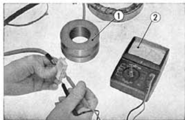
Fig. 8-8 ① Field coil ② Tester
