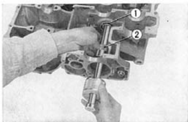
Fig. 5-8 ① Countershaft bearing ② Bearing puller
