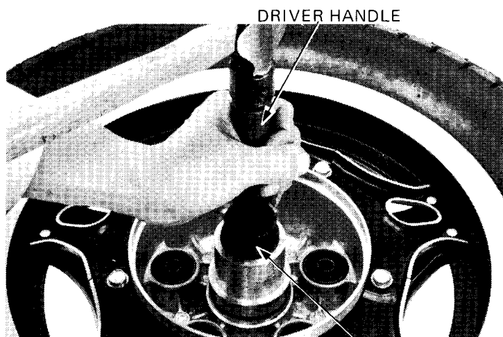
DRIVER HANDLE BEARING DRIVER 62 x 68 mm DRIVER PILOT 20 mm
