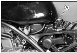
• Pull the fuel tap outlet hose [A] and vacuum hose [B] off the tap.
