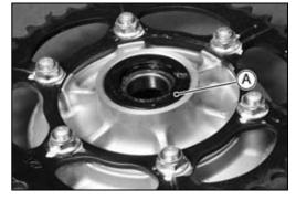
• Remove the bearing by tapping from the brake drum side.
