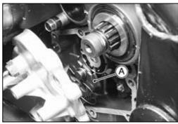
Remove the nut [A] and take off the gear positioning lever
