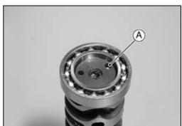
• Install the shift drum cam aligning its groove [A] with the dowel pin [B].
