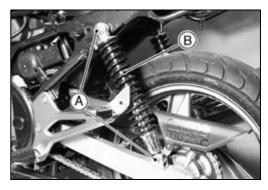
• Remove the mounting bolts [A] and Battery Case [B].
