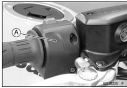
• Free the idle adjusting screw [A] from the bracket.
