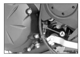
• Loosen the exhaust pipe manifold holder nuts [A].
