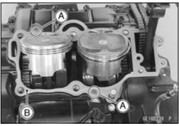
The piston ring openings must be positioned as shown in the figure. The openings of the oil ring steel rails must be about 30 ~ 40° of angle from the opening of the top ring.
