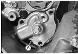
Using the oil pump sprocket bolt [A], pull out the oil pump
