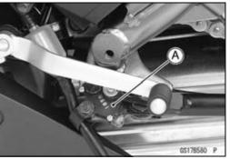
★If the sidestand switch operation does not work, inspect or replace the following item.
