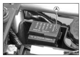
Pull the fuses [A] straight out of the fuse box with needle nose pliers.
