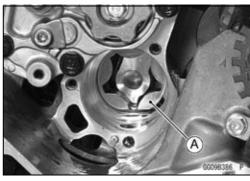
• Remove the oil pump cover [A].
