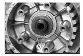
• Replace the clutch hub nut [A] with a new one.
