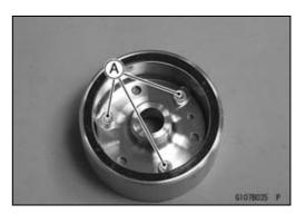
Remove: Starter Motor Clutch [A]
