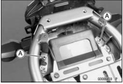
• Remove the tail/brake light mounting bolts [A], and take off the tail/brake light unit [B].
