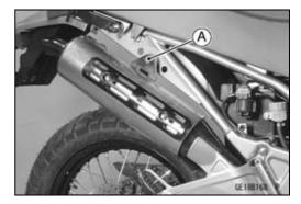
• Remove the exhaust pipe holder nuts [A].
