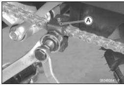
• After staking, measure the outside diameter [A] of the link pin and link plates width [B].
