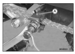
• Using the chain joint "ZJ" tool [A], stake the link pin ends projecting from the plate after aligning the adjusting pin with the "B" mark on the U type holder.
