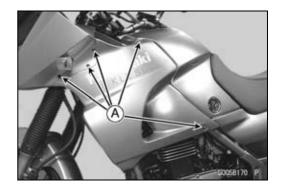
Pull the rear side [A] of the fairing a little to outside to clear the stoppers [B] and then remove the fairing pushing [C] it to forward.
