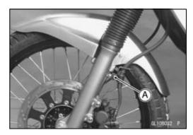
• Remove the brake hose clamp bolts [A] at steering stem.
