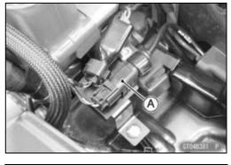
Disconnect the KIBS hydraulic unit connector (see KIBS)  $(\mathbf{B})$ Hydraulic Unit Removal in the Brakes chapter). • Check the wiring continuity of the BK/O lead and W/G
