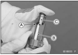
• Turning the tensioner body clockwise, slide the stopper [A] into the groove [B] of the push rod [C].
