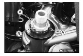
• Adjust the steering using the steering stem nut wrench [A].
