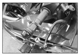
• Tighten the front caliper mounting bolt [A] [B] following specified tightening sequence.
