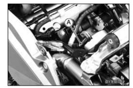
OTo maintain the correct fuel/air mixture (F/A), there must be no intake air leaks in the DFI system. Be sure to install the oil filler plug [A] after filling the engine oil.
