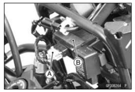
• Fit the slit [A] on the damper to the bracket projection [B] (Both Sides).
