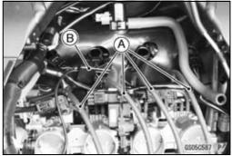
Plug the air switching valve hose end [A] and air cleaner housing fitting [B].
