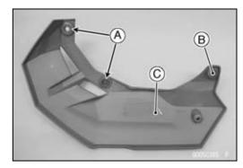
• When installing the grommets [A], position the thick side to the inside.
