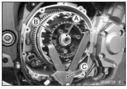
• Install the friction plates [A] and steel plates [B] alternately as shown.
