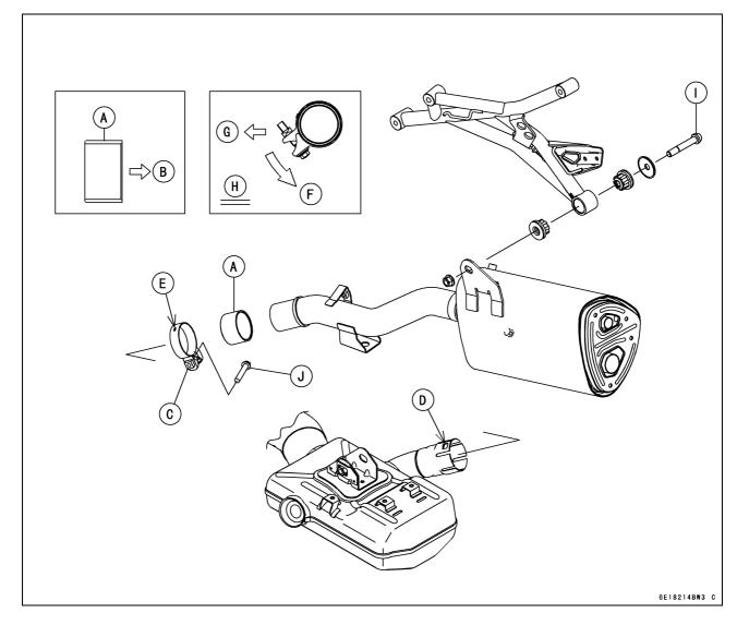
• Thoroughly warm up the engine, wait until the engine cools down, retighten all the bolts and nuts.
