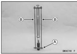
• Screw in the nuts [A] until the piston rod nut comes out.
