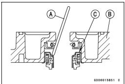
• Take the oil seal [A] out of the housing [B] with a hook [C].
