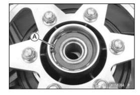
Remove the bearing [A] by tapping from the wheel side.
