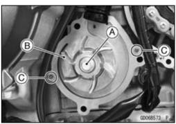
• Remove the water pump housing [A] while pushing the oil pump shaft [B].
