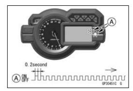
When Registered Ignition Key is Inserted.
