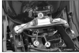
Remove: Fuel Tank Bolts [A]
