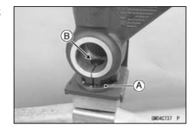
• While holding the top plug [A], insert the fork spring stopper [B] between the piston rod nut [C] and the slider.
