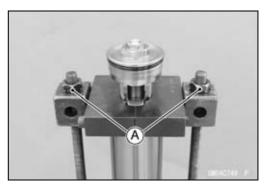
• While holding up the top plug [A], insert the fork spring stopper [B] between the piston rod nut [C] and the slider.
