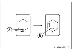
OThe nuts can be tightened by using a torque angle gauge [A].
