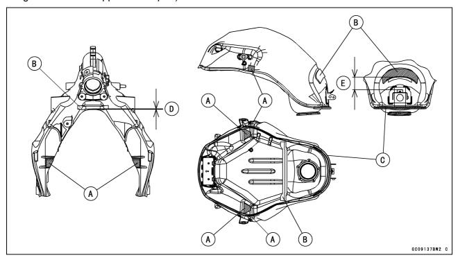
• Put the clean cloth [A] to prevent damage to the frame and brake pipes.
