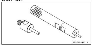
Valve Spring Compressor Adapter,  $\phi$ 24: 57001-1586
