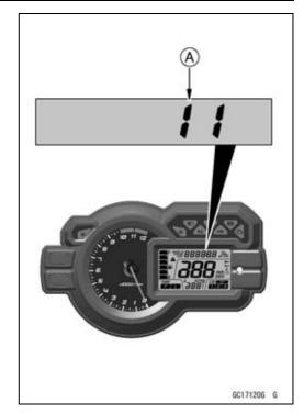
When the service code [A] is displayed, for first ask the rider about the conditions [B] of trouble, and then start to determine the cause [C] of problem.
