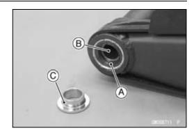
Screw the swingarm pivot adjusting collar [A] into the frame [B] so that the collar does not project the swingarm mating surface [C].
