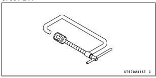
Piston Pin Puller Assembly: 57001-910
