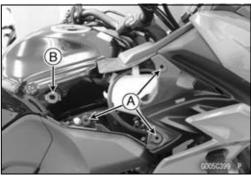
• Insert the projections [A] of the fuel tank cover into the grommets [B].
