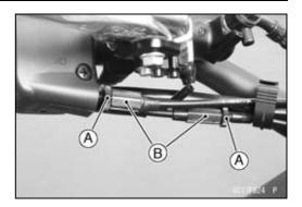
• Remove the adjuster screw [A] from the bracket.
