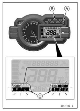
For models equipped with an immobilizer system, the red warning indicator light (LED) [A] and immobilizer warning indicator [B] blink, when a problem occurs in the system.
