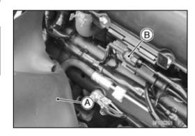
• Clear the crankshaft sensor lead from the band [A] and clamps [B].
