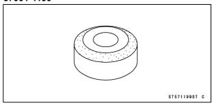
Valve Seat Cutter Holder,  $\phi$ 4.5: 57001-1330
