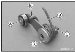
• While prying the gear positioning lever [A], tighten the gear positioning lever bolt [B].
