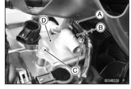
• Remove the air suction valve [A] on both sides.
