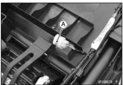
• Connect the key registration unit [A] and key registration adapter [B] as shown.
