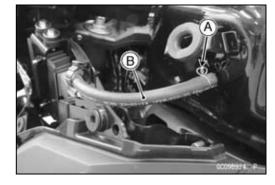
Clear the left side tab [A] of the fuel tank from the meter cover [B] first, and then clear the right side tab of the fuel tank.
