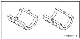
Fork Oil Seal Driver Attachment,  $\phi$ 36 ~ $\phi$ 46: 57001-1798
