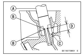
• Ream the valve guide with valve guide reamer [A], even if the old guide is reused.
