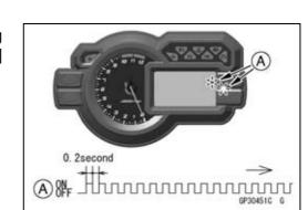
When Registered Ignition Key is Inserted.
