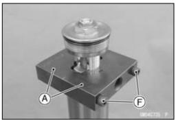
• Set the spring compressor [A] and suitable jack [B] as shown.
