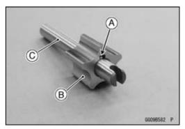
• Turn the pump shaft so that the slot [A] in its shaft fits onto the projection [B] of the pump drive gear shaft.
