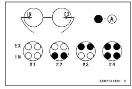
★If the valve clearance is not within the specified range, first record the clearance, and then adjust it.
