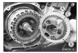
• Install the last friction plate so that the tangs [A] fit into the grooves in the housing as shown.
