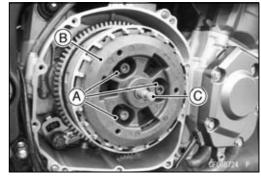
Hold the sub clutch hub [A] steady with the clutch holder [B], and remove the nut [C] and washers.
