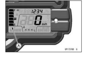
★If the display function does not work, replace the meter assembly.
