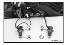
OThe red warning indicator light (LED) and immobilizer warning indicator [A] blink 1 time and stops for 1 second and repeats this cycle.
