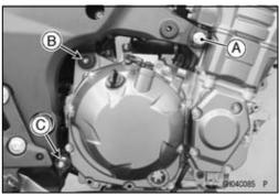
• Using the nut wrench [A], loosen the upper adjusting collar locknut [B].
