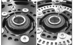
• Apply a thin coat of grease [A] to the front axle [B] for rust prevention.
