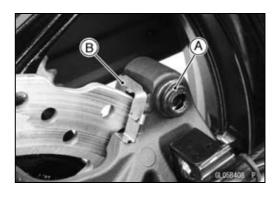
• Fit the rear brake pads [A] to the guide [B].
