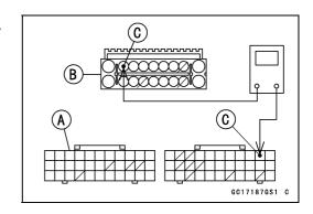
Wiring Continuity Inspection ABS Hydraulic Unit Connector [A]  $\leftarrow \rightarrow$ Front Wheel Rotation Sensor Connector [B]
