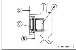
Apply a non-permanent locking agent to the oil passage plugs [A], and tighten them.
