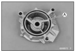
• Be sure to install the dowel pins [A].
