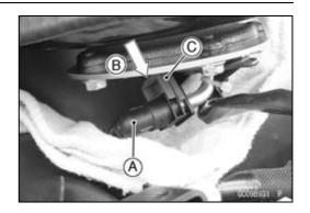
Push and pull [A] the hose joint [B] back and forth more than two times, and make sure it is locked does not come off.
