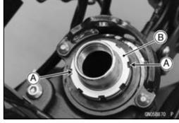
• Pushing up the stem base, and remove the steering stem nut [A] and stem cap [B].
