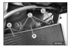
Insert the upper right mounting bracket [A] to the frame projection [B].
