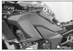
• Pull the side cover [A] outward to clear the projections [B] from the grommets on both sides.
