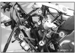
• To remove the ball bearing outer races [A] pressed into the head pipe [B], insert a bar [C] into the recesses [D] of head pipe, and applying it to both recess alternately hammer it to drive the race out.
