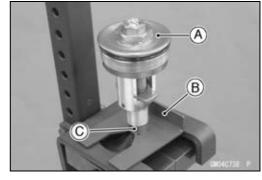
• Holding the top plug [A] with a wrench [B], loosen the piston rod nut [C].
