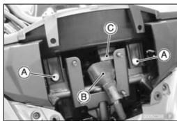
Remove (Both Sides): Quick Rivet [A]
