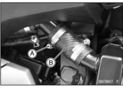
Remove: Cap [A] Radiator Bolt (Upper) [B]
