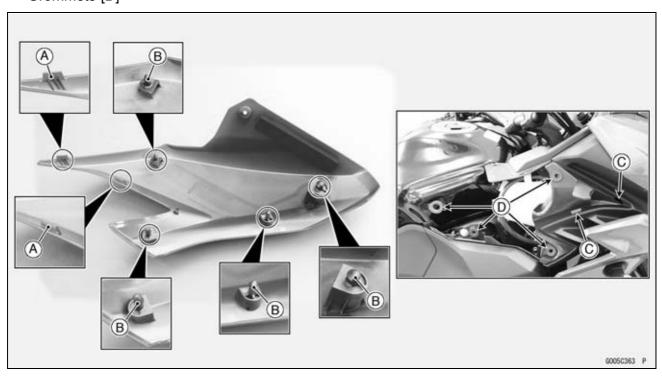
Remove: Fuel Tank Cover Bolt [A] and washer
