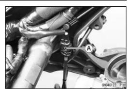
• Remove the connector [A] from the bracket on the air suction valve cover and disconnect the connector.
