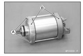
• Remove the armature [A] from the commutator side.
