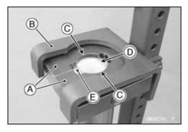
• While holding up the piston rod puller, insert the fork spring stopper between the piston rod nut and the holder.
