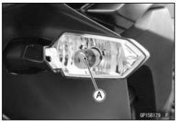
Insert the new bulb [A] by aligning its pins [B] with the grooves [C] in the socket, and turn the bulb clockwise.
