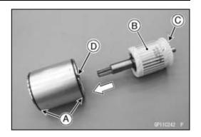
• Install the end cover [A] so that the stopper [B] is aligned with the hollow [C] of the yoke.
