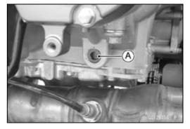
Attach the adapter [A] and gauge [B] to the plug hole.
