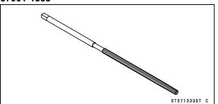
Valve Seat Cutter, 60° -  $\phi$ 33: 57001-1334
