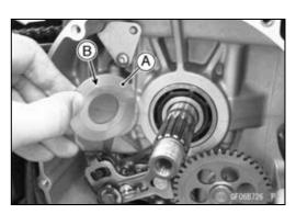
• Engage the clutch housing gear [A] and oil pump drive gear [B] with the crankshaft primary gear [C] and oil pump drive gear [D].
