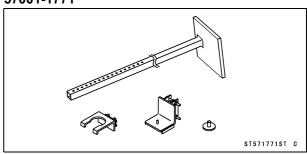
Fork Oil Seal Driver Weight,  $\phi$ 26 ~ $\phi$ 46: 57001-1795
