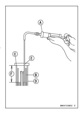
Screw the rod nut [A] onto the piston rod [B] as shown.
