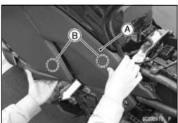
• Put the clean cloth [A] to prevent damage to the frame.
