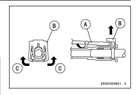
• Pull [A] the fuel hose joint [B] out of the outlet pipe.
