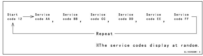
Olf there is no fault, the yellow ABS indicator light (LED) blinks as shown.
