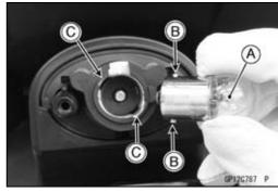
• Insert the holes [A] into the projection [B].
