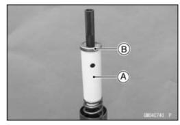
Check the distance between the bottom end [A] of the top plug and rebound damping adjuster [B] with a pair of vernier caliper (Right Front Fork Only).
