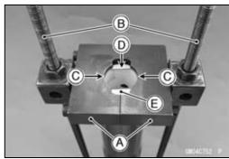
• While holding up the piston rod puller, insert the fork spring stopper between the piston rod nut and the clamp.
