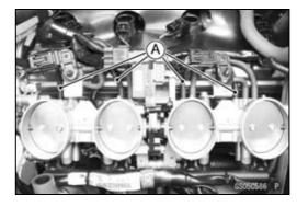
• Connect a vacuum gauge and hoses [A] (Special Tool: 57001-1369) to the fittings on the throttle body.
