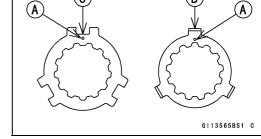
• Fit the steel balls into the 5th gear holes in the output shaft, aligning the holes as shown.
