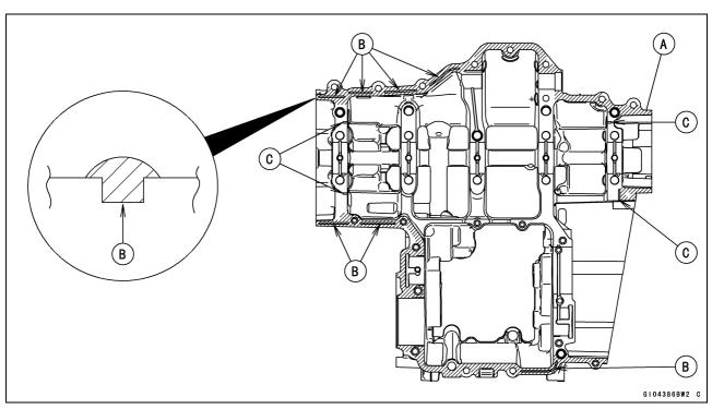
• Fit the lower crankcase to the upper crankcase.
