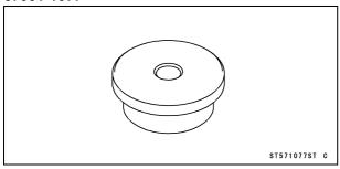
Steering Stem Bearing Driver,  $\phi$ 42.5: 57001-1344
