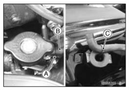
• Remove the radiator cap, and install a cooling system pressure tester [A] on the filler neck.
