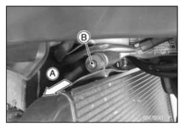
Clear the heat insulation rubber plate [A] from the radiator
