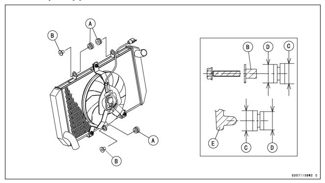
Cover the heat insulation rubber plate [A] on the radiator [B] as shown.
