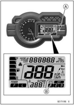
OPush the upper meter button [A] to display the odometer.
