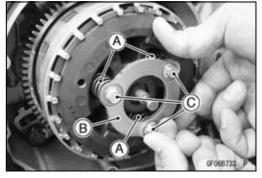
• Tighten the three clutch stopper bolts [A] alternately with little by little (1/4 turn at a time) to prevent tilting the clutch stopper plate [B].
