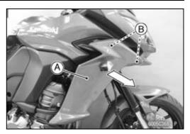
• Disconnect the turn signal light lead connector [A], and remove the middle fairing.
