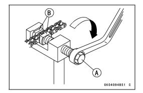
• Set the plate holder (B) [A] and cutting and riveting pin [B] as shown.
