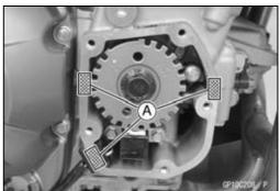
• Replace the O-ring [A] with a new one.
