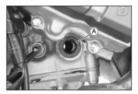
• Install the shift shaft [A] so that the return spring pin [B] fits between the spring [C].
