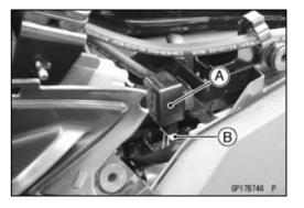
Connect one 12 V battery and turn signal lights as indicated, and count how many times the lights blink for one minute.
