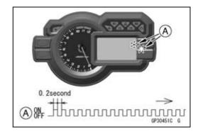
When Registered Ignition Key is Inserted.
