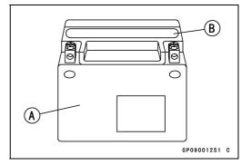
Terminal Voltage: 11.5 ~ less than 12.8 V
