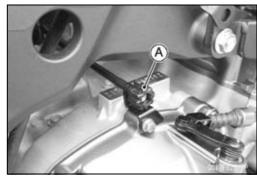
Remove: Throttle Cable Holder Clamp [A] Throttle Cable Lower Ends [B]
