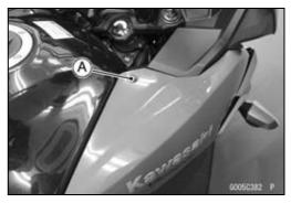
Clear the hooks [A] of fuel tank cover [B] outward while pushing them.
