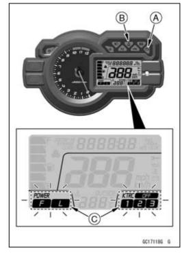
OWhen a problem occurs with immobilizer system (equipped models), the red warning indicator light (LED) [A] and immobilizer warning indicator [B] blink.
