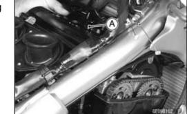
• Remove the cylinder head cover [A] to backward floating it a little up.
