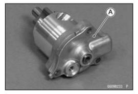
• Remove the outer rotor [A] for feed pump.
