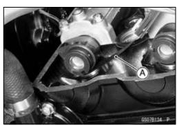
OEach piston has two intake and two exhaust valves. Measure these two intake or exhaust valves at the same crankshaft position.
