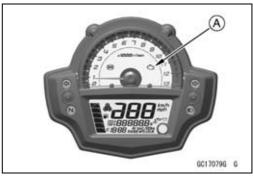
OPush the left meter button [A] to display the odometer.
