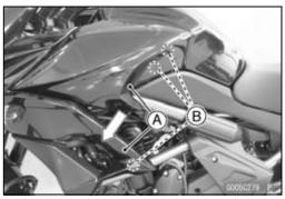
• Clear the hook [A] and tab [B] of the middle fairing from the inner cover [C].
