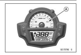
With the engine stopped and turned in the self-diagnosis mode, the service code [A] is displayed on the LCD (Liquid Crystal Display) by the number of two digits.
