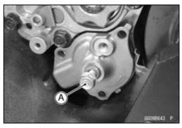
• Using the oil pump sprocket bolt [A], pull out the oil pump [B] as a assembly.
