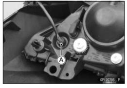
• Pull out the bulb [A] straight from the socket.
