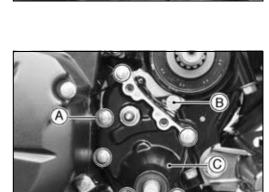
• Remove the shift shaft assembly [A].
