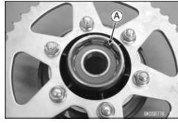
Remove the bearing [A] by tapping from the wheel side.
