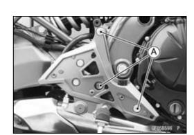
• Remove the exhaust pipe holder nuts [A].
