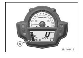
★If the display function does not work, replace the meter assembly.
