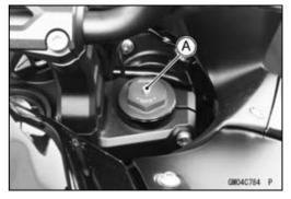
OThe damping force can be left soft for average riding. But it should be adjusted harder for high speed riding or riding with a passenger. If the damping feels too soft or too stiff, adjust it in accordance with the following table.
