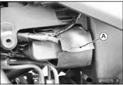
• Pull out the main fuse (30 A) [A] from the starter relay with needle nose pliers.
