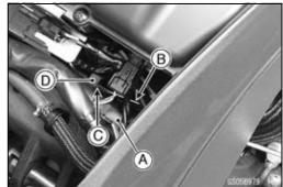
• Pull the fuel hose joint [A] out of the delivery pipe.
