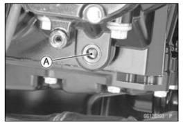
Attach the adapter [A] and gauge [B] to the plug hole.
