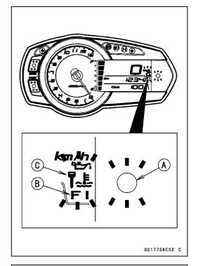
With the engine stopped and turned in the self-diagnosis mode, the service code [A] is displayed on the LCD (Liquid Crystal Display) by the number of two digits.
