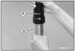
• Remove the inner tube guide bushing [A], outer tube guide bushing [B], washer [C], oil seal [D] from the inner tube.
