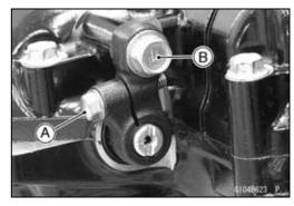
Remove the upper crankcase bolts following the specified sequence.
