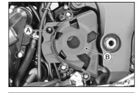
• Remove the engine sprocket outer cover screws [A] to sparate the outer and inner cover [B].
