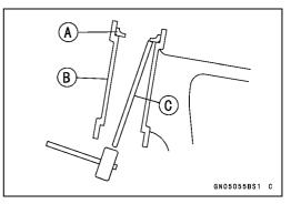
• Remove the lower ball bearing inner race (with its oil seal) [A] which is pressed onto the steering stem with a suitable commercially available chisel [B].
