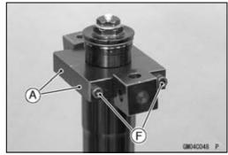
• Insert the holder bar [A] into the axle hole of the front fork [B].
