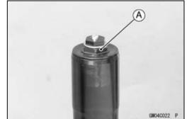
• Holding the top plug [A] with a wrench [B], tighten the spring preload adjuster [C].
