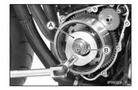
• Using the flywheel puller [A], remove the alternator rotor [B] from the crankshaft.
