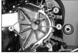
• Remove the speed sensor bolt [A].
