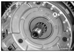
• Install the washer [A] so that the "OUTSIDE" mark [B] faces outward.
