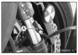
• Insert the hook portions [A] into the slits [B] on the upper fairing (Both Sides).
