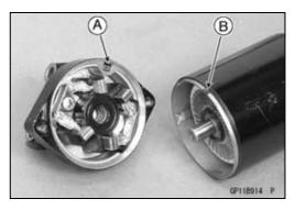
Align the marks [A] to assemble the yoke and the end cover [B].
