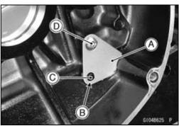
• Press and insert the fitting [A] in the upper crankcase [B] until it is bottomed.
