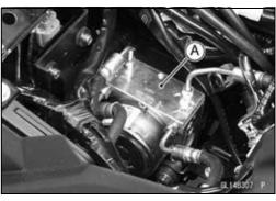
Fuse Box 1 [A] (ABS Fuses and Accessory Fuse)
