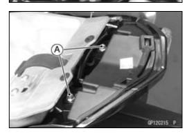
• Disconnect the tail/brake light lead connector [A] to remove the tail/brake light (LED).
