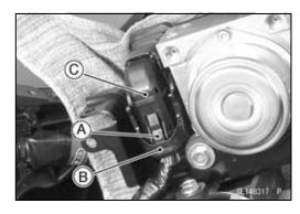
Remove: Bolts [A] ABS Hydraulic Unit [B]
