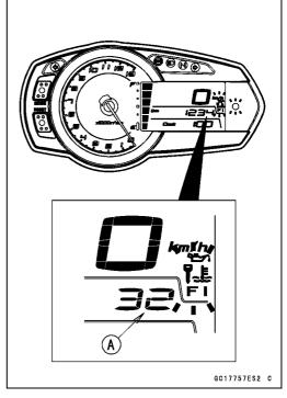
When the service code [A] is displayed, for first ask the rider about the conditions [B] of trouble, and then start to determine the cause [C] of problem.
