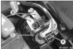
• Connect the hand tester [A] and 12 V battery [B] to the starter relay [C] as shown in the figure.
