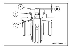
• Set the fork spring compressor on the slider [A] using the outer tube as a guide.
