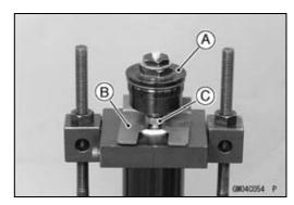
• Holding the spring preload adjuster [A] with a wrench [B], loosen the piston rod nut [C].
