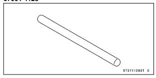
Valve Seat Cutter, 32° -  $\phi$ 33: 57001-1199
