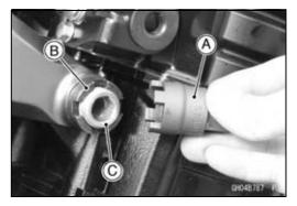
• Using the nut wrench [A], loosen the lower adjusting collar locknut [B].
