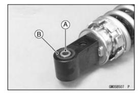
• Remove the needle bearing [A], using the bearing remover head [B] and bearing remover shaft [C].
