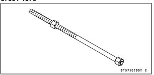
Head Pipe Outer Race Driver,  $\phi$ 54.5: 57001-1077
