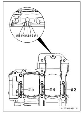
Select the proper bearing insert [A] in accordance with the combination of the crankcase and crankshaft coding.
