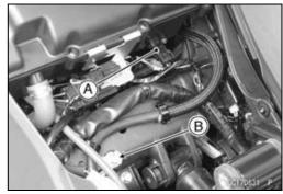
Exhaust Butterfly Valve Actuator [A] Battery 12 V 8 Ah [B] Vehicle-down Sensor [C] FI Fuse 15 A [D]
