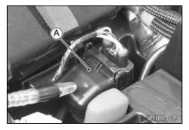
Disconnect: Connector [A] Cable Terminals [B]
