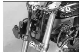
Olf fork leg is to be disassembled, loosen the upper and lower front fork clamp bolts to lower the fork leg [A] as shown. And retighten the lower front fork clamp bolts. Then, loosen the top plug beforhand.
