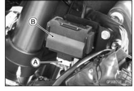
• Fit the slits [A] on the damper to the bracket projections [B].
