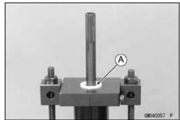
• While holding up the piston rod puller, insert the fork spring stopper between the piston rod nut and the slider.
