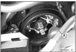
• Fit the dust cover [A] firmly onto the bulb so that the TOP mark [B] is aligned with the arrow mark [C] on the headlight.
