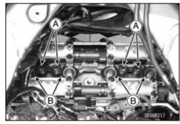
• Apply liquid gasket [A] to the cylinder head as shown.
