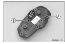
• Separate the meter assembly [A] and upper meter cover [B].
