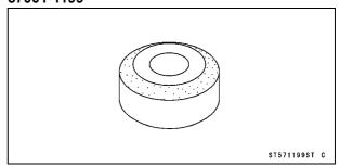
Valve Seat Cutter Holder,  $\phi$ 4.5: 57001-1330
