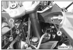
• For left lower fairing installation, insert the stopper [A] into the damper [B] on the left lower side fairing.
