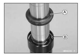
OHolding the outer tube [A] by hand, pull the inner tube [B] several times to pull out the outer tube.
