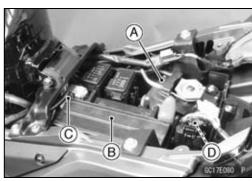
Relay Box (ECU Main Relay, Radiator Fan Relay, Fuel Pump Relay) [A]
