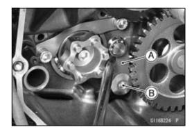
• Install the shift shaft [A] so that the return spring pin [B] fits between the spring [C].
