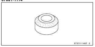
Valve Seat Cutter, 45° -  $\phi$ 32: 57001-1115
