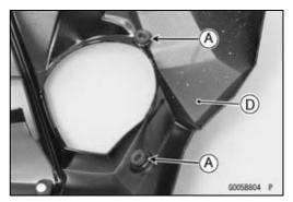
• Connect the turn signal light lead connector [A] (Both Sides).
