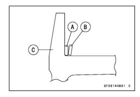
Install the friction plates and steel plates, starting with a friction plate and alternating them.
