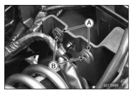
• The UP mark [A] of the sensor should face upward.
