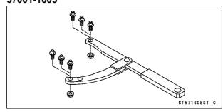
Flywheel Puller Assembly, M38  $\times$  1.5/M35  $\times$  1.5: 57001-1615
