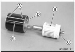
• Align the stopper [A] and hollow [B] to assemble the yoke and end cover.
