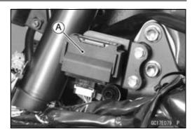
Intake Air Temperature Sensor [A] Frame Ground [B]
