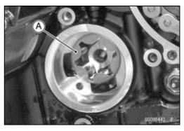
Assemble the pin [A], inner rotor [B] and oil (water) pump shaft [C].
