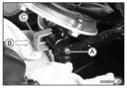
Push and pull [A] the hose joint [B] back and forth more than two times, and make sure it is locked and does not come off.
