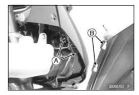
• Insert the stoppers [A] into the dampers [B] on the lower fairing (Both Sides).
