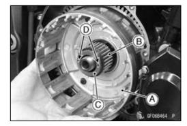
Install the following parts to the drive shaft.
