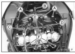
Water Temperature Sensor [A] Speed Sensor [B] Engine Ground [C]
