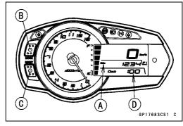
OThe hour display [A] starts flashing.
