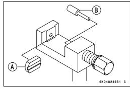
• Turn the pin holder until riveting pin touches link pin.
