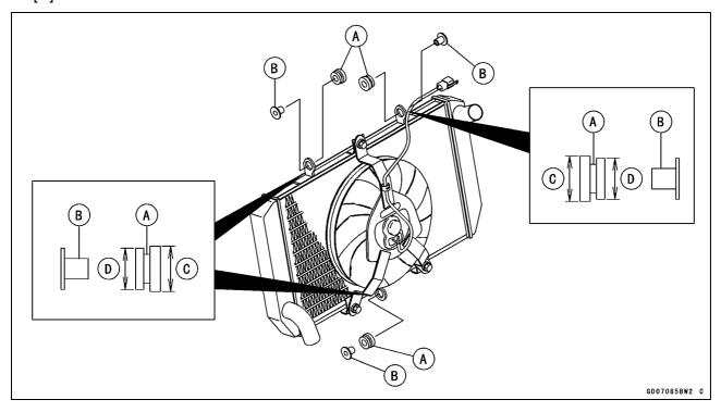
• Fit the slits [A] of the heat insulation rubber plate to the upper mounting brackets [B] and fan bracket [C] as shown.
