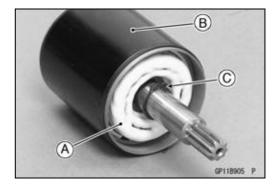
• Remove the starter motor terminal locknut [A].
