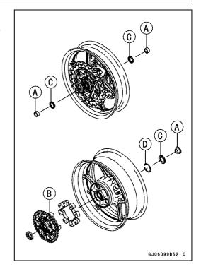
• Use the bearing remover to remove the hub bearings [A].
