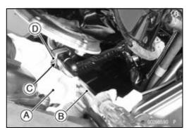
• Pull [A] the fuel hose joint [B] out of the outlet pipe.
