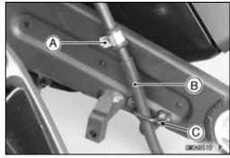
• Unscrew the swingarm pivot shaft nut [A].
