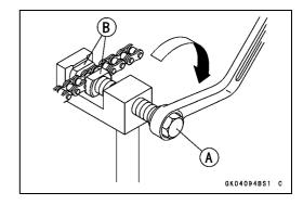
• Set the plate holder (B) [A] and cutting and riveting pin [B] as shown in the figure.
