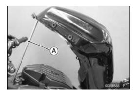
• Remove the drain hose [A] and clamp from the fuel tank.
