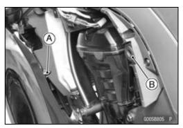
• For right lower fairing installation, insert the damper [A] into the projection [B] on the rear lower fairing.
