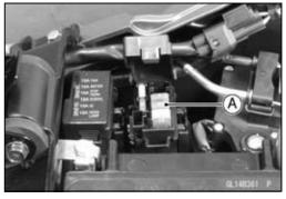
★ If the fuse is good, check the wiring continuity that relates to the R lead in the main harness referring to the ABS System Wiring Diagram.
