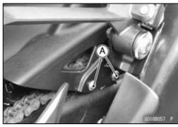
Remove: Quick Rivets [A] Mud Guard [B]
