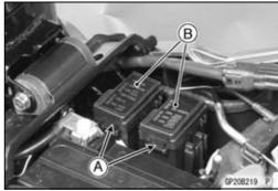
Pull the fuses [A] straight out of the fuse box with needle nose pliers.
