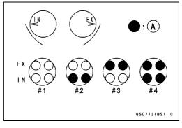
OWhen positioning #1 piston TDC at the end of the compression stroke:
