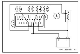
Check that the segments number of the fuel level gauge [A] matches the resistance value of the variable rheostat.
