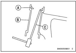
Remove the lower ball bearing inner race (with its oil seal)
