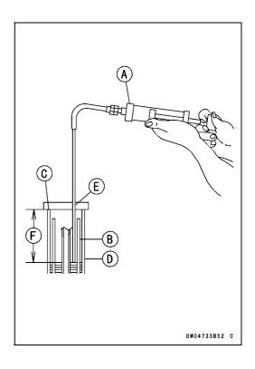
Screw on the rod nut [A] fully to the piston rod [B].
