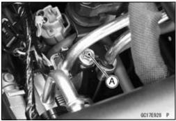
• Disconnect the vacuum hose [A], and remove the rubber damper [B] from the intake air pressure sensor #1 [C].
