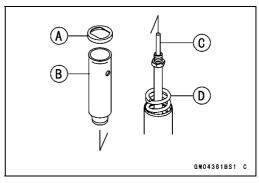
Screw the rod nut [A] onto the piston rod [B] as shown.
