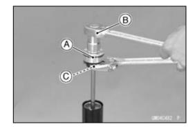
• Using the fork piston rod stopper holder [A], remove the piston rod assy stopper [B].
