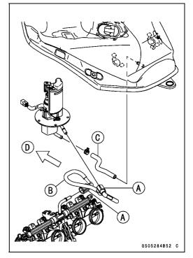
Check that the outlet hose joints are securely connected.
