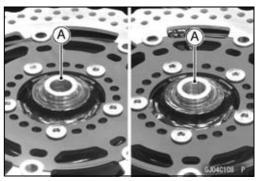
Before tightening the axle clamp bolt [A] on the right front fork leg, pump the front fork up and down 4 or 5 times to allow the right front fork leg to seat on the front axle.
