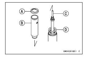
Screw the rod nut [A] onto the piston rod [B] as shown.
