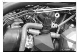
• Install the suitable plugs [A] on the fitting of the air suction valve covers, and shut off the secondary air.
