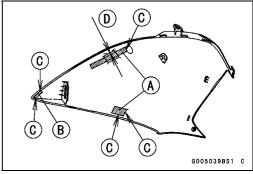
• When installing the hook fasteners [A], align the edge of the hook fasteners with the lines [B] of the fuel tank.
