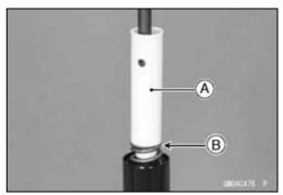
Set the fork spring compressor on the spacer [A].
