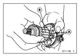
• Align the line marks [A] of the end cover with the square mark [B] on the yoke.
