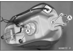
• When installing the dampers [A], position the thick side [B] to frame side [C].
