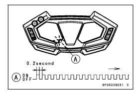
When Registered Ignition Key is Inserted.
