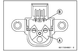
When the motorcycle is down, the ignition switch is left ON. If the starter button is pushed, the electric starter turns but the engine does not start. To start the engine again, raise the motorcycle, turn the ignition switch off, and then on.
