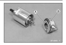
• Remove the terminal locknut [A] and terminal bolt [B], and then remove the brush with the brush plate [C] from the right-hand end cover.
