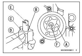
• Fit the pin [A] of the oil pump cover [B] into the hole [C] in the crankcase.
