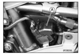
• Pull out the fuses [A] from the starter relay with needle nose pliers.
