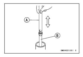
Oil Level (fully compressed, without spring) Standard:
