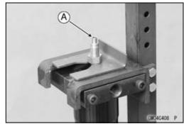
Check the distance between the bottom end [A] of the top plug and rebound damping adjuster [B] with a pair of vernier caliper (Right Front Fork Only).
