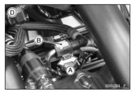
Check that the intake hose [A] is onto the pipe fully and the clamps [B] are installed beyond the raised rib [C].
