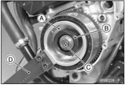
Using the flywheel puller [A], remove the alternator rotor
