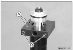
• Set the spring compressor [A] and a suitable jack [B] as shown.
