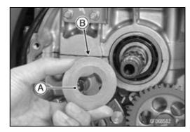
Olnstall the spacer [A] so that the "OUTSIDE" mark [B] faces outward.
