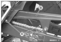
• Unscrew the swingarm pivot shaft locknut [A], using the nut wrench [B].
