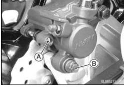
Remove: Pad Pin [A] Brake Pads [B]
