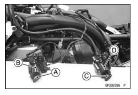
OThe red warning indicator light (LED) and immobilizer warning symbol [A] blink 1 time and stops for 1 second and repeats this cycle.
