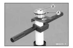
• Holding the top plug [A] with a wrench [B], tighten the piston rod nut [C] against the top plug.
