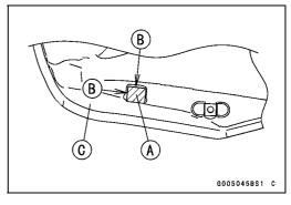
• Check that the pad [A] is in place on the middle fairing [B].
