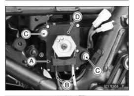
• Remove the pulley bolt while holding the pulley [A] with the suitable tool [B].
