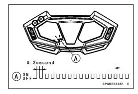
When Registered Ignition Key is Inserted.
