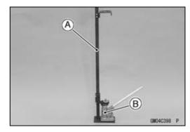
• Insert the projection of the protector [A] into the front fork bottom hole [B].
