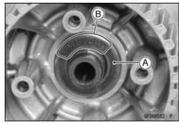
OReplace the clutch hub nut with a new one.
