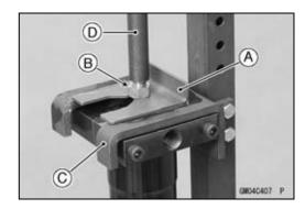
• Install the rebound damping adjuster rod [A] (Right Front Fork Only).
