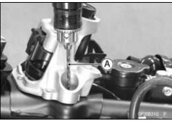
• Remove the ignition switch bolts [A] to separate the ignition switch [B] and bracket [C].
