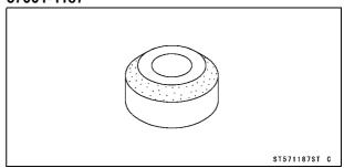
Valve Spring Compressor Adapter,  $\phi$ 21: 57001-1272
