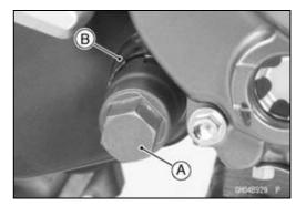
Using the Hexagon Wrench, turn the lower adjusting collar [A] counterclockwise to make the gap between the engine and lower adjusting collar.
