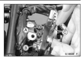
Remove: Bolt [A] ABS Hydraulic Unit Assembly [B]
