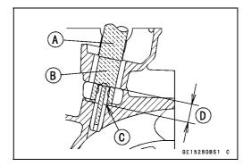
• Ream the valve guide with valve guide reamer [A], even if the old guide is reused.
