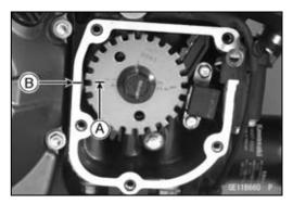
• Using the thickness gauge [A], measure the valve clearance between the cam and the valve lifter.
