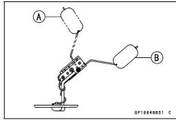
• Using the hand tester [A], measure the resistance across the terminals in the fuel level sensor lead connector [B].
