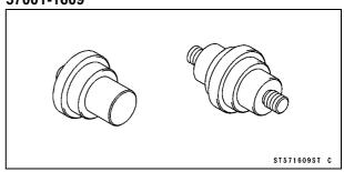
Needle Bearing Driver,  $\phi$ 28: 57001-1610
