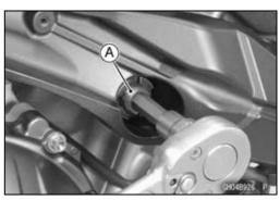
• Remove the left front engine mounting bolt [A].
