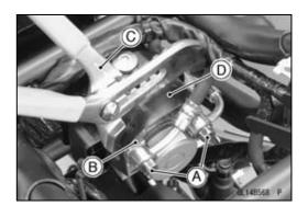
• Remove the brake hose banjo bolts [A] while holding the ABS hydraulic unit [B] with a suitable plier [C].
