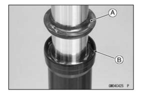
OHolding the outer tube [A] by hand, pull the inner tube [B] several times to pull out the outer tube.
