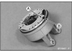
• Install the shim [A] on the armature shaft.
