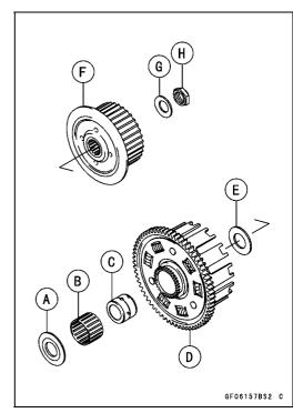
Olnstall the spacer [A] so that the tapered side [B] faces inward.
