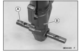
• Insert the lower end of the compression shaft [A] into the hole [B] of the holder bar.
