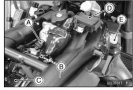
Intake Air Temperature Sensor [A]
