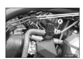
• Install the suitable plugs [A] on the fitting of the air suction valve covers, and shut off the secondary air.
