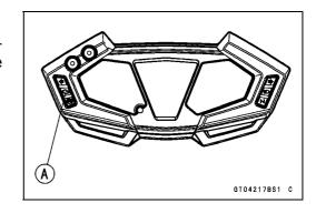
When a problem occurs with immobilizer system, the red warning indicator light (LED) [A] blinks and immobilizer warning symbol [B] is displayed on the LCD, when a problem occurs in the system.
