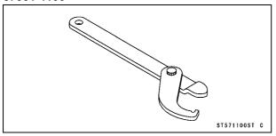
Steering Stem Bearing Driver,  $\phi$ 42.5: 57001-1344
