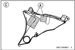
• When installing the grommet [A], face the thick side toward the inside [B] of the left frame cover [C].
