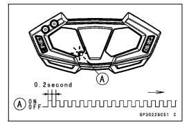
When Registered Ignition Key is Inserted
