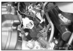
Remove: Screws [A] Right Switch Housing [B]
