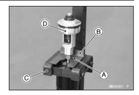
Holding the piston rod nut with a wrench [A], remove the top plug [B] from the piston rod.
