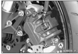
Remove: Pad Pin [A] Brake Pads [B]
