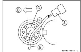
• Pull the joint lock [A] fully as shown.
