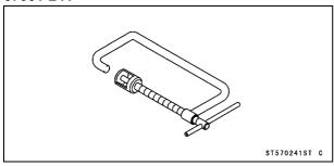
Piston Pin Puller Assembly: 57001-910
