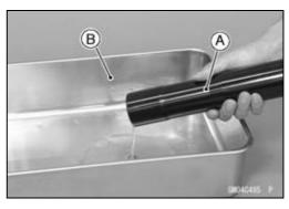
• Insert the holder bar [A] into the axle hole of the front fork [B].
