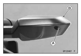
Push and turn the bulb [A] counterclockwise and remove it
