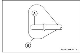
• Install a new fuel intake hose [A] so that the white mark side [B] faces outlet pipe [C] of the fuel tank.
