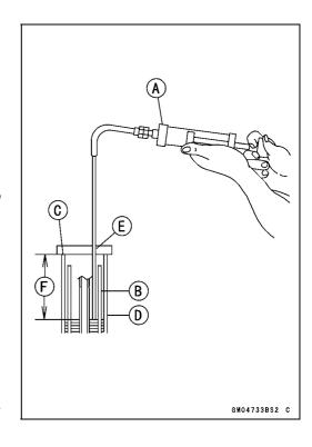
Screw the fork piston rod puller onto the end of the piston rod.
