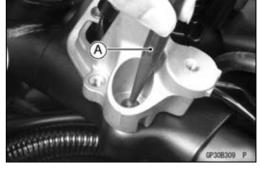
ullet Extend the punch mark with the  $\phi 2$  mm drill [A]. In addition, extend the punch mark with the  $\phi 3.5$  mm drill. Lastly, shave off the Torx bolt head with the  $\phi 6.5$  mm drill.
