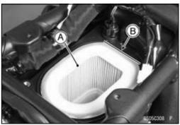
• ZR800A/B Models, when installing the pad [A], align the edge of the pad with the rib [B] of the air cleaner duct.
