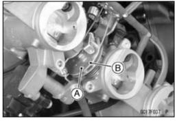
• Install the throttle body assy holder clamp bolts in the direction as shown.
