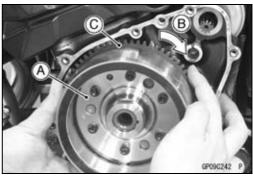
• Using a cleaning fluid, clean off any oil or dirt on the washer [A] and dry it with a clean cloth.
