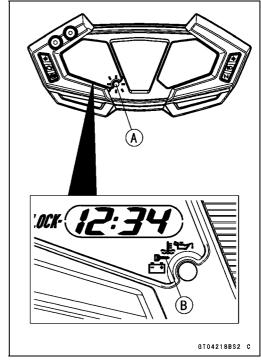
With the engine stopped and turned in the self-diagnosis mode, the service code [A] is displayed on the LCD (Liquid Crystal Display) by the number of two digits.
