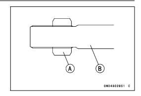
Screw the fork piston rod puller onto the end of the piston rod.
