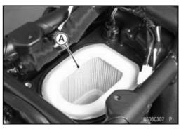
• Install a new element [A] so that flat side [B] faces forward.
