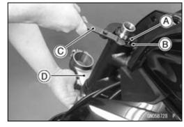
To remove the ball bearing outer races [A] pressed into the head pipe [B], insert a bar [C] into the recesses of head pipe, and applying it to both recess alternately hammer it to drive the race out.
