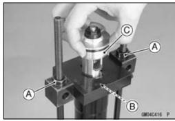
Insert the fork spring stopper [A] between the piston rod nut [B] and the clamp [C] while holding up the top plug [D].
