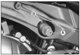
Using the Hexagon Wrench, turn the upper adjusting collar [A] counterclockwise to make the gap between the engine and upper adjusting collar.
