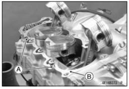
• The piston ring openings must be positioned as shown.
