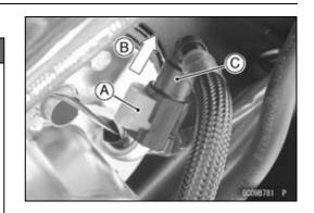
• Pull [B] the fuel hose joint [C] out of the fuel outlet pipe.
