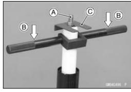
Remove: Spacer [A] Fork Spring [B]
