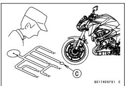
Even when the DFI system is operating normally, the yellow engine warning indicator light (LED) goes on may be displayed under strong electrical interference. Additional measures are not required. Turn the ignition switch off to stop the indicator light.
