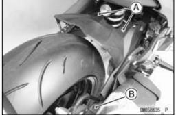
To adjust the spring preload, turn in the adjusting nut to the desired position and tighten the locknut by using hook wrenches [A] with the rear shock absorber attached the frame.
