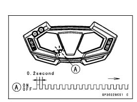
When Registered Ignition Key is Inserted.
