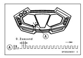
When Registered Ignition Key is Inserted.
