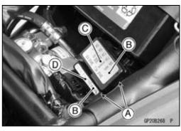
• Pull the fuses [A] straight out of the fuse boxes with needle nose pliers.
