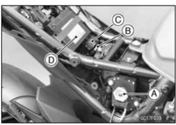
Relay Box [A] (ECU Main Relay, Radiator Fan Relay, Fuel Pump Relay) ECU [B] Immobilizer/Kawasaki Diagnostic System Connector [C]
