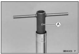
Take the cylinder unit [A] out of the inner tube [B].
