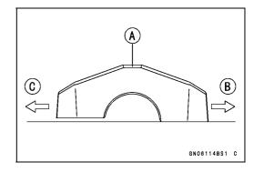
• When installing the lower handlebar holders, install the upper handlebar holder [A] and handlebar holder bolts [B] temporarily as shown.
