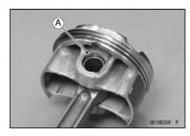
Using the piston pin puller assembly [A], remove the piston pin.
