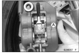
• Install the brake pads [A] on the pad spring correctly. OFit the pad into the groove of the caliper.
