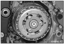
Set the special tools as shown to hold the clutch stopper plate.
