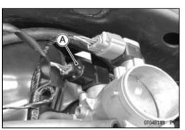
Connect the setting adapter [A] between the harness connector and main throttle sensor connector.
