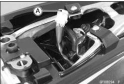
Connect the key registration unit [A] and key registration adapter [B] as shown.
