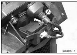
Oxygen Sensor [A] (Equipped Models)
