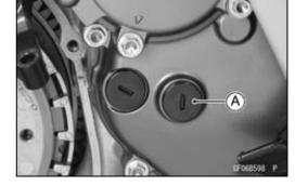
Using a wrench on the starter clutch bolt, turn the crankshaft clockwise until the clutch stopper bolts [A] reaches the position as shown.
