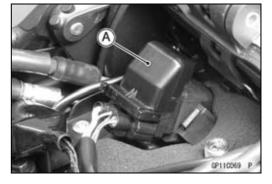
Pull out the fuses [A] from the starter relay with needle nose pliers.
