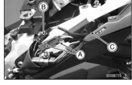
Remove: Flap Mounting Bolts [A] Clamp [B] Flap
