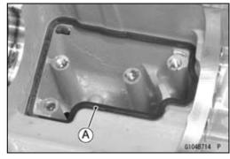
OApply a non-permanent locking agent to the threads of the bolts [A] and tighten them.
