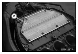
Install a new element [A] so that the screen side [B] faces upward.
