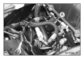
OTo maintain the correct fuel/air mixture (F/A), there must be no intake air leaks in the DFI system. Be sure to install the oil filler plug [A] after filling the engine oil.
