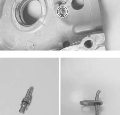
• Apply engine oil to the new O-ring and install it.
