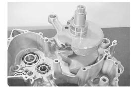
Remove the crankshaft.
