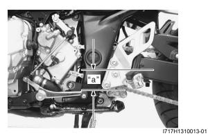
Adjust the drive chain slack. Refer to "Drive Chain Inspection and Adjustment in Section 0B (Page 0B-17)".
