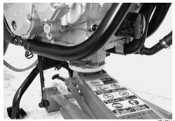
28) Remove the engine mounting bracket (25).
