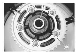
• Remove the rear sprocket mounting drum retainer ?.
