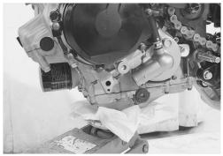
• Remove the engine mounting bolts (A) and (C).
