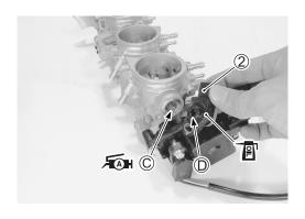
• Apply thin coat of engine oil to the new O-rings 3 and cushion seals 4.
