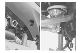
• Install the muffler chamber and mufflers . ( 6-16)
