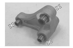
• Remove the cushion lever bearings with the special tool.
