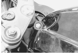
• Lift and support the fuel tank with the fuel tank prop stay.
