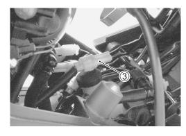
Connect proper lead wires to the fuel pump lead wire coupler (fuel pump side) and apply 12 V to the fuel pump (between Y/R wire and B/W wire) for 10 seconds and measure the amount of fuel discharged.
