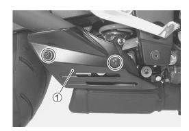
Loosen the muffler chamber connecting bolt. (LH/RH)
