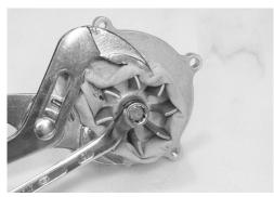
• Remove the mechanical seal ring ⑦ and rubber seal ⑧ from the impeller.
