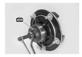
• First install the right wheel bearing, then install the left one with the special tools.
