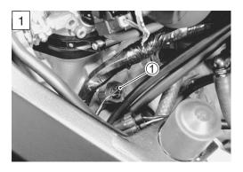
DATA ECT sensor voltage: 4.5 – 5.5 V
