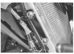
Disconnect the water/air bleed hose ① and radiator inlet hose
