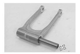
• Remove the cushion rod bearings with the special tool.
