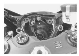
• Disconnect the steering damper solenoid valve coupler ①.
