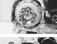
Install the clutch cover and tighten its bolts to the specified torque.
