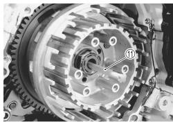
• Unlock the clutch sleeve hub nut.
