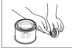
• Install the wheel bearings with the special tools as follows.
