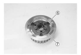
• Install the spring washers ®, clutch lifter driven cam 9 and clutch lifter drive cam 10 to the clutch sleeve hub 7.
