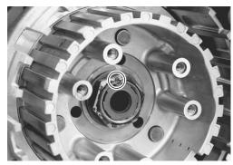
• Install the spring washer seat ③ and spring washer ④ onto the clutch sleeve hub correctly.
