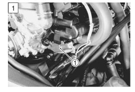
4) Disconnect the secondary injector coupler and measure the resistance between terminals.
