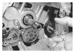
• Install the oil pump drive gear ① to the primary driven gear assembly ②.
