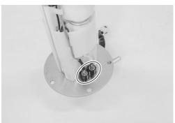
• Remove the fuel level gauge 1.
