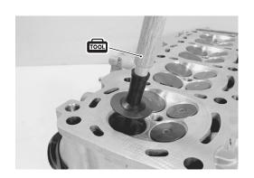
seat width is not uniform, reface the seat using the seat cutter.
