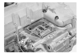
• Remove the oil filter with the special tool.
