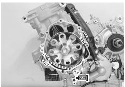
Install the dowel pins and new gasket ①.
