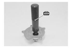
• Apply a small quantity of the grease to the oil seal lip.
