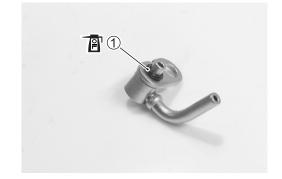
• Install each piston cooling oil jet with the bolt.
