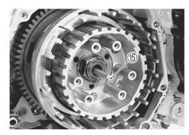
• Install the clutch push piece ®, bearing ® and thrust washer ® to the countershaft.
