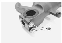
• Remove the damper rod bolt with the special tool.
