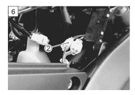
3) Apply 12 V to the terminals and check the operation of EXCVA.
