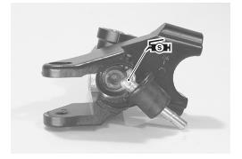
Apply SUZUKI SILICONE GREASE to the bushing and clutch lever pivot bolt.
