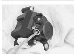
• Remove the dust seal 7 and piston seal 8.
