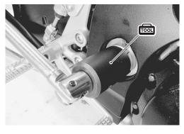
• Hold the swingarm pivot shaft ④ and remove the swingarm pivot nut ⑤.
