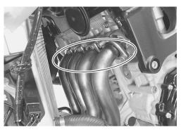
• Remove the exhaust pipe gaskets 11.
