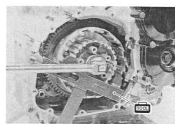
Remove the wave washer ① washer ②, clutch sleeve hub ③ and washer.
