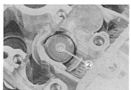
Using special tools, compress the valve springs and remove the two cotter halves 3 from valve stem.
