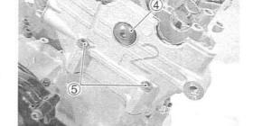
· Remove the cylinder head bolts and washers.
