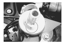
Install the steering stem lock-nut and tighten it to the specified torque with the special tools.
