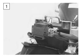
5) Measure the resistance between terminal (A) and terminal (C).
