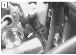
TP sensor input voltage: 4.5 – 5.5 V
