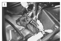
4) Disconnect the HO2 sensor coupler and measure the resistance between terminals.
