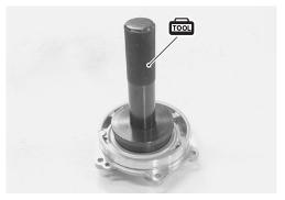
Remove the driveshaft left bearing dust seal from the retainer using the special tool.
