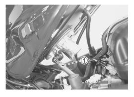
Install the special tools between the fuel tank and fuel delivery pipe.
