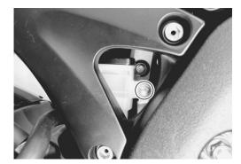
• Loosen the rear shock absorber bracket.
