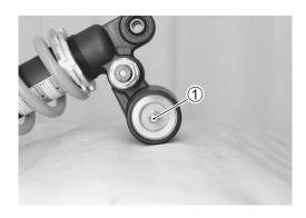
· Press the valve with a screwdriver to bleed out the nitrogen gas.
