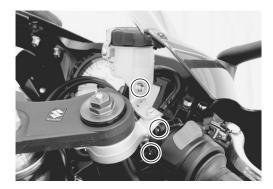
• Remove the reservoir cap ③, insulator ④, diaphragm ⑤ and reservoir tank ⑥.
