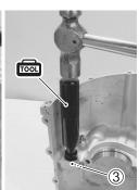
• Install new oil seal with the special tool.
