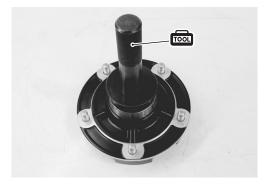
• First install the right wheel bearing, then install the left wheel bearing with the special tools.
