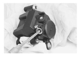
• Remove the dust seal 7 and piston seal 8.
