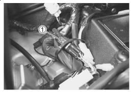
Check the resistance between the terminals of the HO2 sensor.
