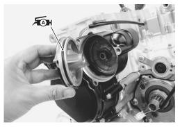
• Install the starter idle gear cover and tighten its bolts to the specified torque.
