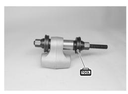
• Apply SUZUKI SUPER GREASE "A" to the bearings, spacers.
