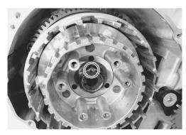
• Hold the clutch sleeve hub with the special tool.
