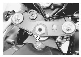
• Insert the protrusion (A) of the handlebars into the hole (B) of the steering stem upper bracket.
