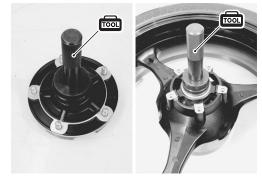
• Apply SUZUKI SUPER GREASE "A" to the dust seal lip before assembling rear wheel.
