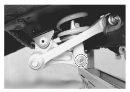
• Remove the rear shock absorber.
