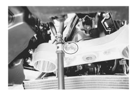
• Remove the steering stem lock-nut, washer and steering stem nut with the special tools.
