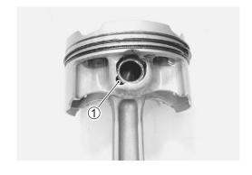
• Separate the piston and conrod by driving out the piston pin.
