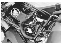
• Remove the rear shock absorber upper and lower mounting bolts and nuts.
