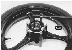
• Remove the wheel bearings with the special tool.
