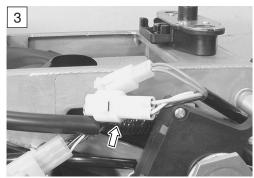
6) Disconnect the position sensor coupler and measure the resistance. (between Y and W wires)
