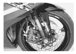
• Tighten two axle pinch bolts on the left front fork leg to the specified torque.
