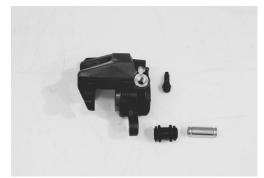
• Place a rag over the piston to prevent it from popping out and then force out the pistons using compressed air.
