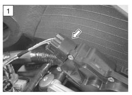
4) Turn the ignition switch ON to check the STV operation. (STV operating order: Full open  $\rightarrow$  95% open)
