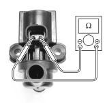
If the resistance is not within the standard range, replace the PAIR control solenoid valve with a new one.
