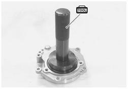
Install the driveshaft left bearing dust seal with the special tool.
