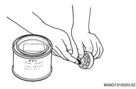
Install the bearing (1) and dust seal (2) to the sprocket mounting drum with the special tools.
