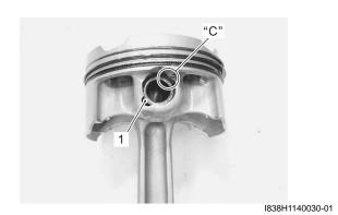
• Apply a small quantity of molybdenum oil solution to the sliding surface of the pistons and cylinder walls.
