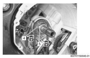
• Install the clutch assembly. Refer to "Clutch Installation in Section 5C (Page 5C-7)".
