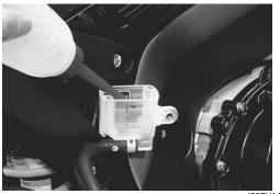
5) Fill the reservoir with new brake fluid.
