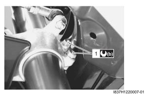
6) Tighten the front fork upper clamp bolt (3).
