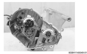
• Install the clutch push rod oil seal retainer (4).
