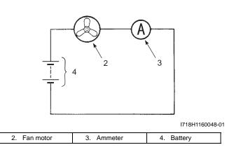
3) Connect the cooling fan motor coupler.
