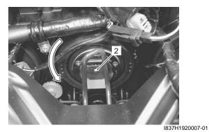
4) Replace the headlight bulb (Low beam) with a new one.
