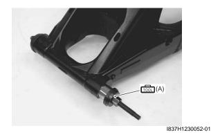
3) Apply grease to the bearings.
