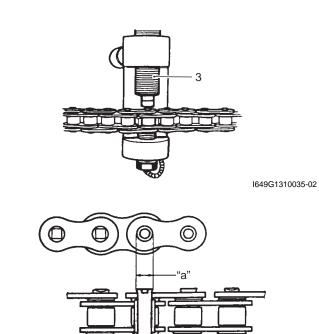
Adjust the drive chain slack, after connecting it. Refer to "Drive Chain Inspection and Adjustment in Section 0B (Page 0B-15)".
