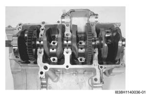
4) Apply engine oil to each crank pin and bearing surface.
