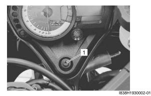
2) Disconnect the coupler (2) and remove the combination meter assembly.
