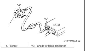
Using a test male terminal, check the female terminals of the circuit being checked for contact tension.
