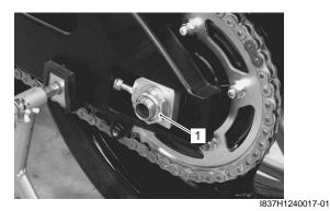
4) Remove the rear wheel by disengaging the drive chain.
