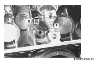
Insert the valve, with its stem coated with molybdenum oil solution all around and along the full stem length without any break.
