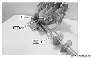
2) Remove the gearshift shaft oil seal (2). (LH only)
