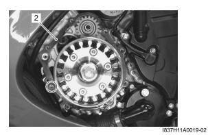
• Apply grease to the starter motor O-ring.
