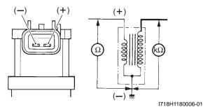
3) After measuring the ignition coil/plug cap resistance, reinstall the removed parts.
