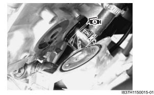
• Apply a small quantity of thread lock to the oil cooler mounting bolts and tighten them to the specified torque.
