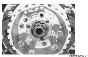
12) Hold the clutch sleeve hub with the special tool.
