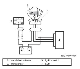
Also, when the ignition switch is turned ON, the indicator light flashes as many as the number of IDs registered in ECM. Thereafter, if the IDs are in agreement, the indicator light turns on for two seconds to notify of completion in successful communication. If the indicator light (LED) flashes fast, it notifies of communication error or disagreement of ID.
