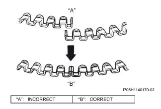
b) Install the 2nd ring (3) and 1st ring (4) to piston.
