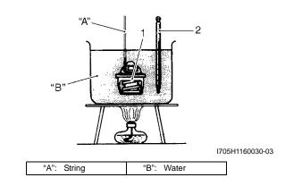
6) Read the thermometer just when opening the thermostat. If this reading, which is the temperature level at which the thermostat valve begins to open, is out of the standard value, replace the thermostat with a new one.
