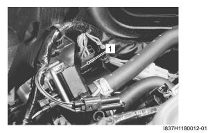
4) Inspect the engine stop switch for continuity with a tester.
