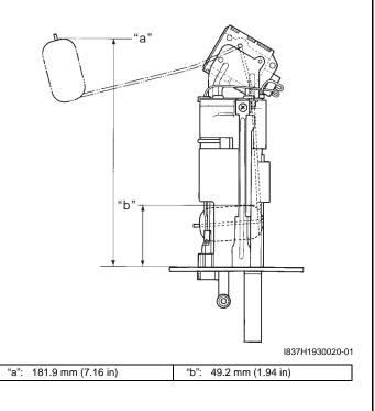
Install the fuel pump. Refer to "Fuel Pump Disassembly and Assembly in Section 1G (Page 1G-11)".
