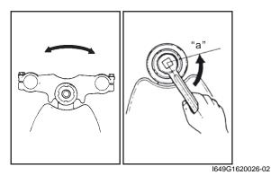
• When installing the washer (2), align the lug of the washer to the groove of the steering stem.
