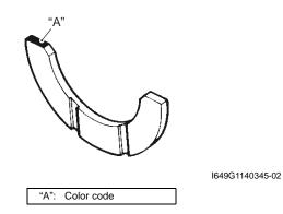
5) After selecting a left-side thrust bearing, install it and then measure the thrust clearance again.
