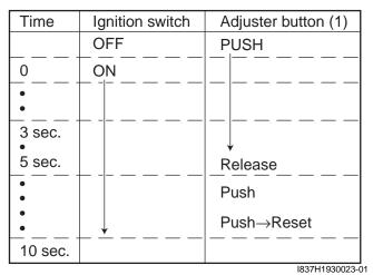
Pointers will return to the proper position right after the completion of the operation. In the case of the pointers not returning to the proper position after doing above, replace the combination meter unit. Refer to "Combination Meter Removal and Installation (Page 9C-2)".
