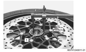
3) Remove the bearings (2) using the special tool.
