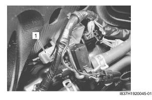
Inspect the dimmer switch for continuity with a tester. If any abnormality is found, replace the left handlebar switch assembly with a new one. Refer to "Handlebar Removal and Installation in Section 6B (Page 6B-2)".
