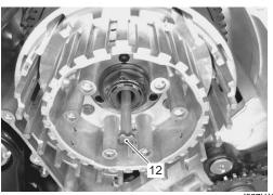
11) Unlock the clutch sleeve hub nut.
