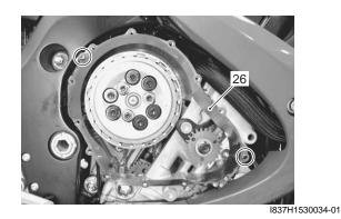
23) Apply a bond lightly to the CKP sensor grommet.
