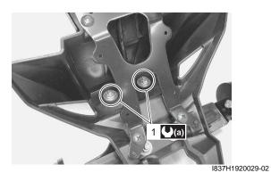
• Apply thread lock to the rear fender (rear) bolts (2) and tighten them.
