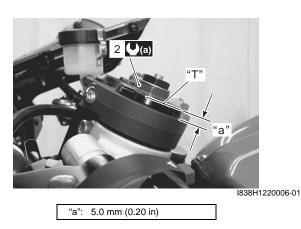
5) Tighten the front fork lower clamp bolts (1).
