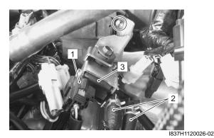
4) Remove the bracket from the EVAP system purge control solenoid valve.
