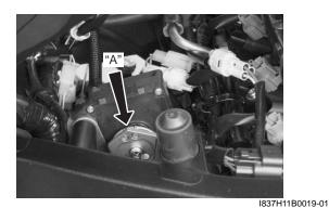
8) Loosen the lock-nut (2) on the No. 2 cable (3) and turn in the cable adjuster (1) fully.
