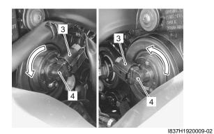
7) Replace the headlight bulb (High beam) with a new one.
