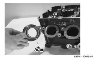
• Install the intake pipes.
