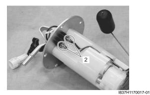
4) Remove the fuel level gauge (3).
