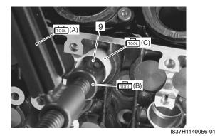
• Be sure that the rounded lip "F" of the cotter fits snugly into the groove "G" in the stem end.
