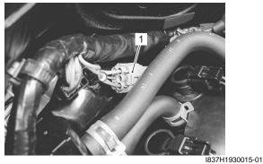
3) Inspect the ignition switch for continuity with a tester. If any abnormality is found, replace the ignition switch with a new one.
