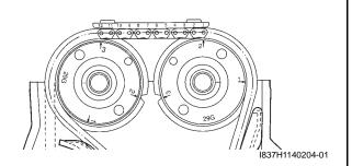
3) Remove the cam chain tension adjuster (2).
