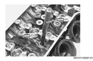
After installing the valve guides, refinish their guiding bores using the reamer. Be sure to clean and oil the guides after reaming.
