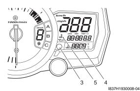
Resistance "A" LED (3) Water temperature LED (4) LED (5) 2.45 k $\Omega$  and more OFF "\_ \_ \_" 19 and below Approx. 0.318 kΩ OFF "80" Approx. 80 °C "120" – "139" 120 – 139 °C 0.1108 kΩ and less ON Flicker 140 °C and over 0 kΩ (Jumper wire) ON "HI" Flicker
