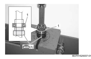
• When installing the gear bushing onto the countershaft, align the shaft oil hole "A" with the bushing oil hole "B".
