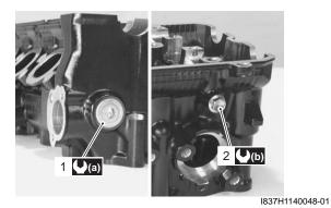
• Apply grease to O-rings of the intake pipes.
