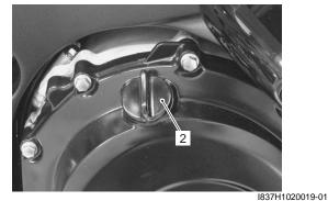
3) Tighten the oil drain plug (1) to the specified torque.
