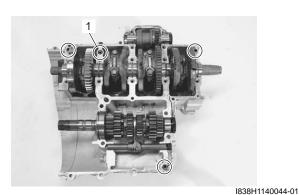
• Apply bond to the mating surface of the lower crankcase as follows.
