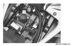
3) First, check for insulation with the tester between terminals "A" and "B". Next, check for continuity between "A" and "B" with 12 V voltage applied, positive (+) to terminal "C" and negative (-) to terminal "D". If continuity does not exist, replace the relay with a new one.
