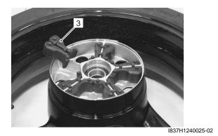
5) Remove the bearings (4) on both sides using the special tool.
