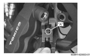
6) Install the new brake pads and pad spring with the pad mounting pins.
