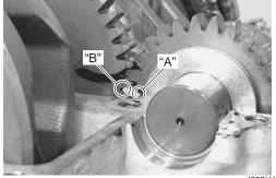
Apply a molybdenum oil solution to each balancer
