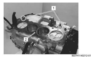
• Place the cylinder head on the cylinder.
