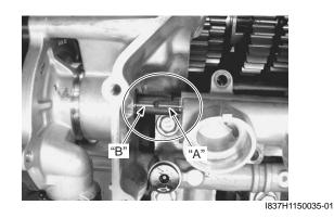
3) Tighten the oil pump mounting bolts to the specified torque.
