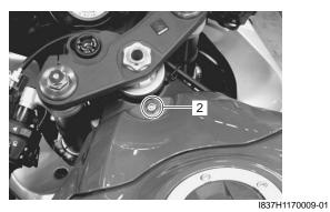
4) Lift and support the fuel tank with the prop stay.
