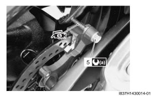
• Set the rubber boot onto the brake caliper and sliding pin.
