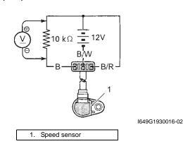
3) Move a screwdriver back and forth across the pickup surface of the speed sensor. The voltage readings should cycle as follows (0 V  $\rightarrow$  12 V or 12 V  $\rightarrow$  0 V). If the voltage reading does not change, replace the speed sensor with a new one.
