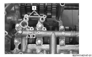
Install the oil pump (2) and tighten the oil pump bolts
