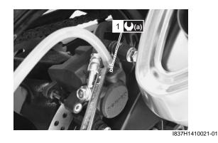
9) Fill the reservoir with brake fluid to the upper mark of the reservoir.
