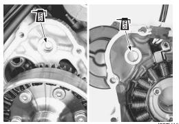
• Apply molybdenum oil solution to the starter idle gear No. 1 shaft holes.
