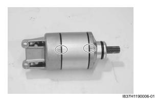
• Tighten the starter motor housing bolts (1) to the specified torque.
