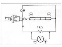
Lift and turn the front wheel and check that voltage varies between 0 - 6 V.
