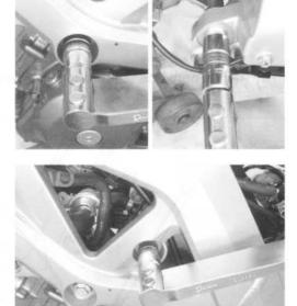
Tighten the engine mounting thrust adjuster locknuts to the specified torque with the special tool.
