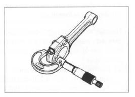
CRANK PIN WIDTH Check the crank pin width (A). Crank pin width Standard: 42.17 – 42.22 mm (1.660 – 1.662 in)
