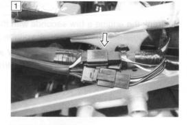
4) Disconnect the CKP sensor coupler ① and measure the resistance.
