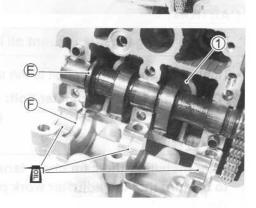
• Tighten the camshaft journal holder bolts to the specified torque.
