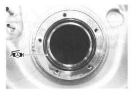
• When installing the fuel pump assembly, first tighten all the fuel pump assembly mounting bolts lightly in the ascending order of numbers, and then tighten them to the specified torque in the above tightening order
