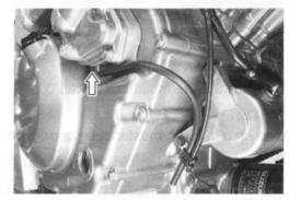
Remove the snap ring and water pump driven gear 3.
