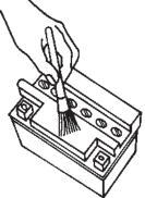
so cleaning materials don't get into cells and neutralize the acid.
