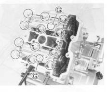
Recheck the rear camshaft positions, intake and exhaust.
