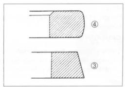
• 1st ring and 2nd ring have letters "T" marked on the side. Be sure to bring the marked side to the top when fitting them to the piston.
