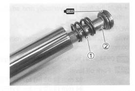
Apply THREAD LOCK to the cylinder bolt and tighten it to the specified torque.
