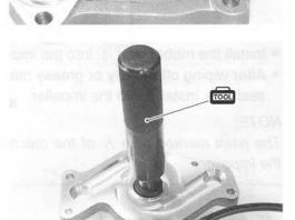
Install the new mechanical seal using the special tool.
