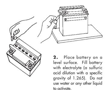
Electrolyte should be between 60°F and 86°F before filling. Fill to UPPER LEVEL as indicated on battery.
