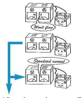
Adjust voltage so that current will be at standard amps after 5 minutes.
