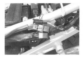
If the peak voltage on the CKP sensor lead wire coupler is ok but on the ECM coupler is out of specification, the wire harness must be replaced. If both peak voltages are out of specification, the CKP sensor must be replaced and re-checked.
