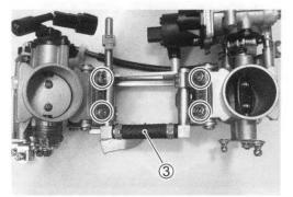
• Remove the throttle link rod ① and secondary throttle link rod ②.
