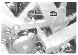
• Tighten all engine mounting bolts or nuts to the specified torque. (23-3-14)
