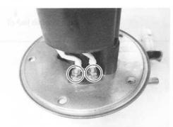
• Remove the screws and fuel level switch.
