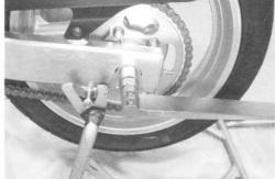
Apply SUZUKI SUPER GREASE to the clutch push rod and install it.
