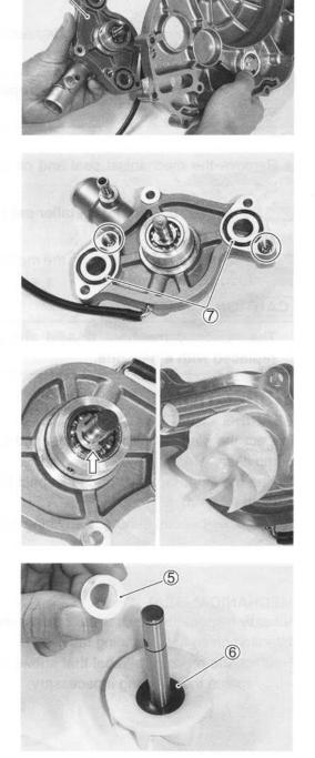
· Remove the bearing using the special tool.
