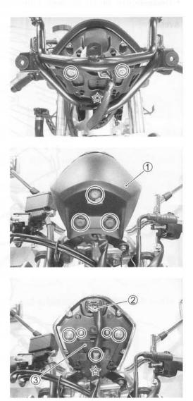
• Disassemble the combination meter as shown in the illustration.
