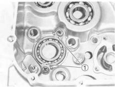
Remove the crankcase bearings by using the special tool.
