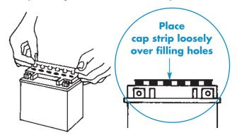
6. Newly activated sealed VRLA batteries require an initial charge. After adding electrolyte, a new battery is approximately 80% charged. Place cap strip loosely over the filling holes as shown in drawing above. Immediately charge your battery after the "stand" period, to bring it to a full state of charge. <u>See</u> "Charging a Newly Activated Sealed VRLA Battery" on page 30.
