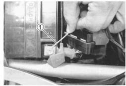
Apply 12 volts to the fuel pump for 10 seconds and measure the amount of fuel discharged.
