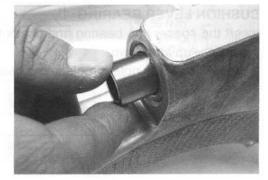
Remove the swingarm pivot bearing and spacer with the special tools.
