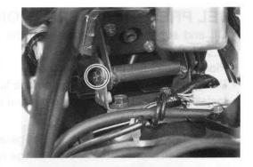
· Remove the fuel tank bracket.
