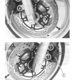
Slightly loosen the front axle by using the special tool.
