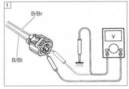
5) If OK, then measure the voltage between B/BI wire terminal and B/Br wire terminal.
