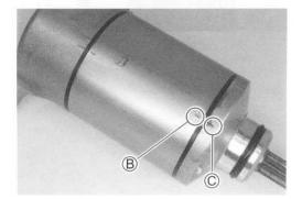
Apply SUZUKI SUPER GREASE to the starter motor O-rings.
