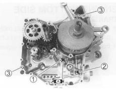
When securing the right and left crankcase halves, tighten each bolt a little at a time to equalize the pressure. Tighten all the securing bolts to the specified torque values.
