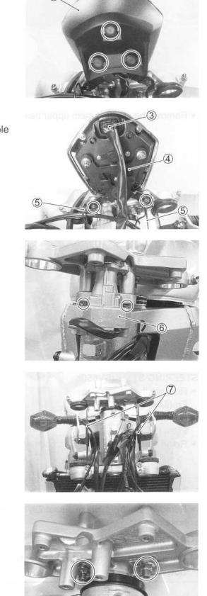
• Remove the steering stem upper bracket by removing the steering stem head nut.
