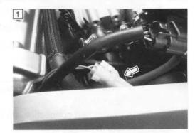
4) Disconnect the PAIR control solenoid valve coupler and measure the resistance between terminals.
