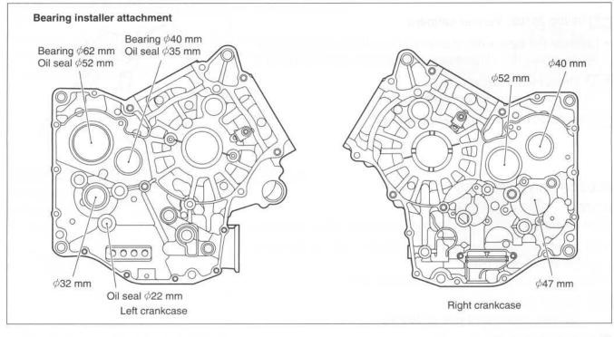
• Apply SUZUKI SUPER GREASE to the oil seal lip.
