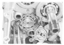
Apply a small quantity of THREAD LOCK to the gearshift cam stopper plate bolt and tighten it to the specified torque.
