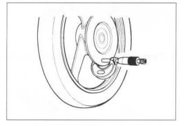
Measure the runout with a dial gauge. Replace the disc if the runout exceeds the service limit.
