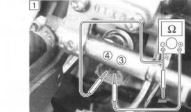
5) If OK, then check the continuity between injector terminals and ground.
