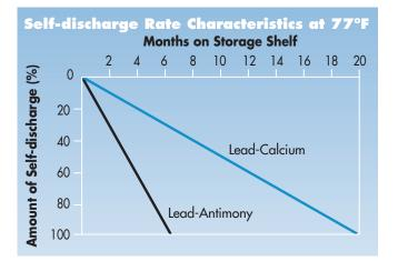
**Self-Discharge:** Self-discharge goes on all the time. It's a battery fact of life that they get weaker from "just sitting." How rapidly batteries self-discharge depends, first of all, on battery type. Lead-calcium batteries, such as YUASA's CX, YT, YI, discharge more slowly than conventional batteries. At room temperature lead-calcium discharges at 1/300 volt per day. Conventional lead-antimony batteries discharge at 1/100 volt per day.
