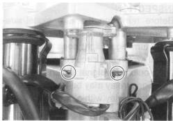
Install the ignition switch in the reverse order of removal.
