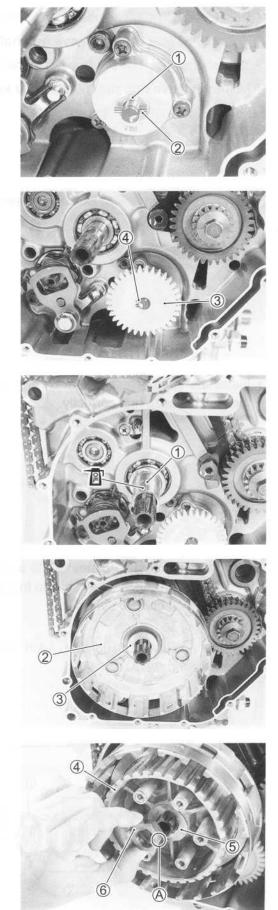
• Hold the clutch sleeve hub with the special tool.
