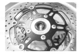
· Remove the dust seal by using the oil seal remover.
