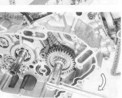
Remove the water pump drive gear ① and primary drive gear ②.
