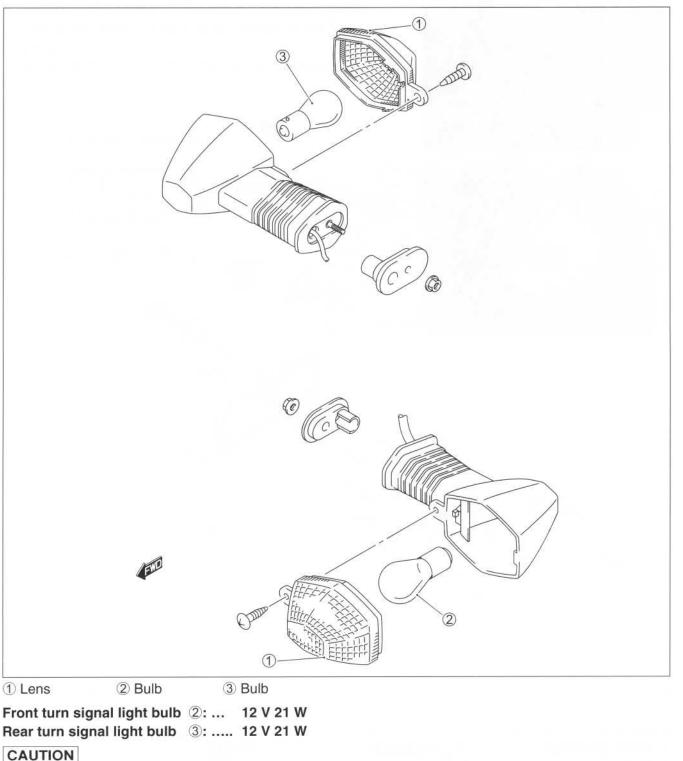
Do not overtighten the lens fitting screws.
