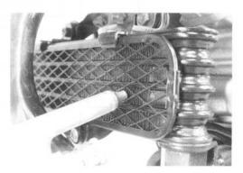
Fins bent down or dented can be repaired by straightening them with the blade of a small screwdriver.
