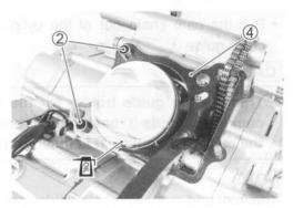
• Apply engine oil to the sliding surface of the cylinders.
