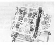
Install the front cylinder head in same manner as the rear cylinder head installation.
