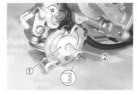
Apply SUZUKI MOLY PASTE to the fast idle link lever.
