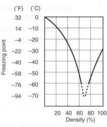
Fig.1 Engine coolant density-freezing point curve.
