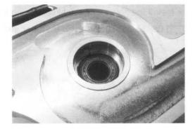
**BEARING CASE** Visually inspect the bearing case for damage. Replace the water pump body if necessary.
