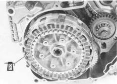
• Install the clutch push rod (2) into the countershaft.
