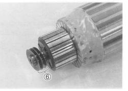
• Install the seal rings (a) to starter motor case (7).
