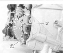
The other arrow mark "2" on the exhaust camshaft sprocket should now be pointing straight up. Starting from the roller pin that is directly above the arrow mark "2" count out 16 roller pins (from the exhaust camshaft side going towards the intake camshaft side). Engage the 16 roller pin D on the cam chain with the arrow mark "3" on the intake sprocket. (23-103)
