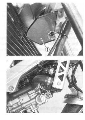
· Remove the radiator lower mounting bolt.
