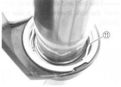
• Pull the inner tube out of the outer tube with light impact.
