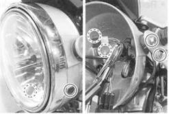
• Remove the speedometer lower cover 2.
