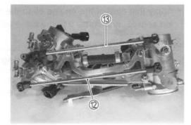
Install the IAP sensor vacuum damper and hose.
