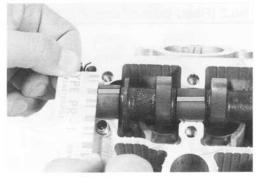
If the camshaft journal oil clearance measured exceeds the limit, measure the inside diameter of the camshaft journal holder and outside diameter of the camshaft journal. Replace the camshaft or the cylinder head depending upon which one exceeds the specification.
