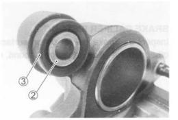
• Remove the spacer ② and boot ③ from the caliper.
