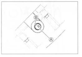
The other arrow mark "2" on the intake camshaft sprocket should now be pointing straight up. Starting from the roller pin that is directly above the arrow mark "2" count out 16 roller pins (from the intake camshaft side going towards the exhaust camshaft side). Engage the 16th roller pin ① on the cam chain with the arrow mark "3" on the exhaust sprocket.
