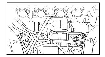
3. Temporarily tighten the bolts (engine bracket 2 and engine) (1) and bolts (engine bracket 2 and frame) 2.
