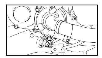
The following procedure applies to all of the coolant drain bolts and copper washers.
