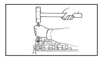
5. To secure the valve cotters onto the valve stem, lightly tap the valve tip with a soft-face hammer.
