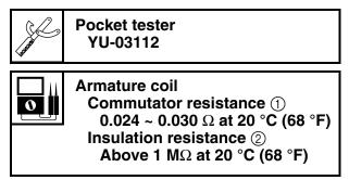
b. If any resistance is out of specification, replace the starter motor.
