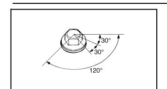
c. Tighten the crankcase bolts further to reach the specified angle 120° in the proper tightening sequence as shown.
