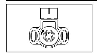
e. Connect the pocket tester ( $\Omega \times 1k$ ) to the throttle position sensor.
