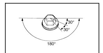
e. Tighten the cylinder head bolts further to reach the specified angle 180° in the proper tightening sequence as shown.
