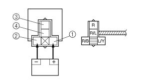
Does the fuel injection system relay have continuity between blue/white and black?
