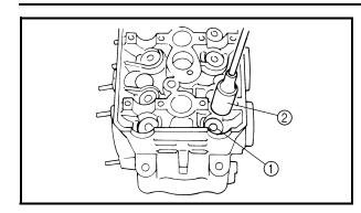
e. Install the new valve pad ① and the valve lifter ②.
