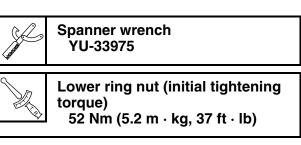
c. Loosen the lower ring nut one turn and then tighten it to specification with a steering nut wrench.
