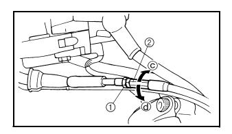
ADJUSTING THE THROTTLE CABLE FREE PLAY/ CHECKING THE SPARK PLUGS
