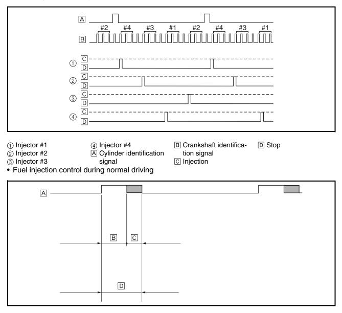
A #1 cylinder fuel injection timing
