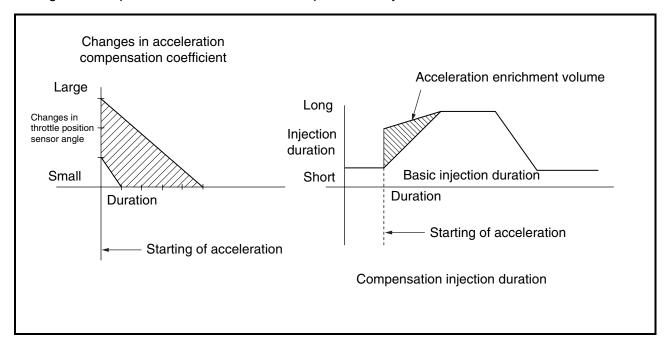
Changes in compensation coefficient and compensation injection duration
