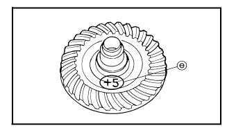
c. To find ring gear shim thickness "B", use the following formula:
