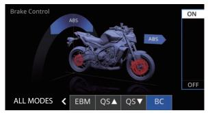
OFF: Only the standard ABS (anti-lock brake system), which adjusts brake pressure based on vehicle speed and wheel speed data. The standard ABS is designed to engage and maximize braking when the vehicle is upright.
