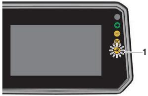
3. After the smart key system indicator light "--®" goes off, use the main switch to enter the smart key identification number "1" located on the identification number card. (Refer to the following procedure on how to input the identification number.)
