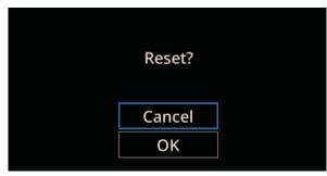
Use this menu to mass reset the multi-function meter to its default settings. This includes YRC settings, display settings, grip warmer presets, traction control, units, Bluetooth connection settings, and vehicle information display items. Confirm by selecting "OK".
