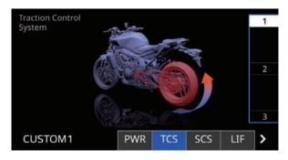
This model uses a variable traction control system. For each setting level, the farther the vehicle is leaned over, the more traction control (system intervention) is applied. There are 3 setting levels available. Level 1 applies the least system intervention, while level 3 applies the most overall traction control to reduce rear wheel slippage.
