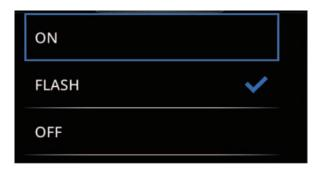
Select "ON" to have the indicator come on at the final r/min. Select "FLASH" to have the indicator start flashing at the initial r/min. When the final r/min is reached, the indicator light will start flashing at a higher frequency. Select "OFF" to turn the indicator off. Short press "\(\sigma\)" to select the highlighted option and return to the previous menu.
