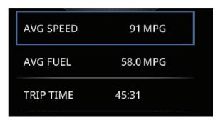
This menu allows reset of the vehicle information display items. Operate the joystick to highlight an item. Short press "✓" to reset the item. Confirm by selecting "OK".
