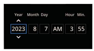
To manually adjust the clock, operate the joystick left-right to highlight an item and up-down to adjust the highlighted item. Short press "✓" to finalize the clock setting and then select "OK" to confirm.
