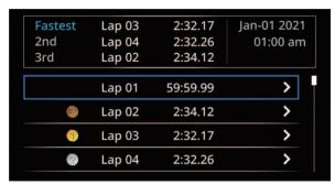
Operate the joystick in the direction of the arrows to access additional lap data and delete lap data individually.
