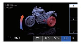
"LIF" can be set to 1, 2, and 3. Setting level 1 provides the least amount of system intervention and setting 3 most strongly reduces the amount of wheel lift.
