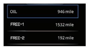
This menu allows you to record distance traveled between engine oil changes "OIL" and two other maintenance items of your choice "FREE-1" and "FREE-2". After maintenance to one of the items has been completed, operate the joystick to highlight the item. Short press "\( \sigma \)" to reset the item. Confirm by selecting "OK". "Vehicle Info"
