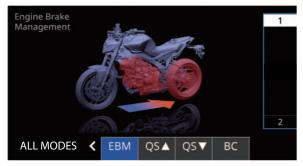
"EBM" can be set to 1 or 2. Setting level 1 provides the least amount of system intervention and setting 2 most strongly reduces engine braking.
