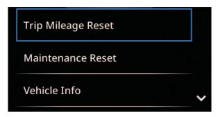
This menu allows the viewing and reset of tripmeters, maintenance tripmeters, vehicle information items, and the mass reset of other settings to factory defaults. "Trip Mileage Reset"
