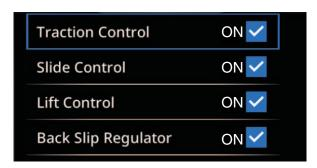
This menu allows you to activate/deactivate the stability control systems: "Traction Control" (TCS), "Slide Control" (SCS), "Lift Control" (LIF), and "Back Slip Regulator" (BSR).
