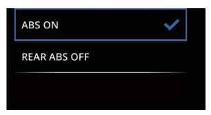
This module allows you to turn the rear wheel ABS (anti-lock braking system) on/off. The currently selected ABS mode is indicated by the REAR ABS OFF indicator "...".
