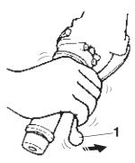
10. After the pulsating action has stopped in the brake lever, it is generated in the brake pedal "1" and continues for a few seconds.
