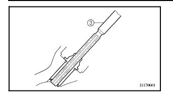
Valve guide remover Intake (4.0 mm, 0.16 in) 90890-04111
