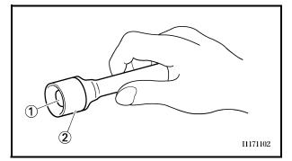
5. To secure the valve cotters onto the valve stem, lightly tap the valve tip with a soft-face hammer.
