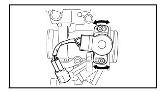
Throttle position sensor resistance 0 ~ 5  $\pm$  1.5 k $\Omega$  at 20 °C (68 °F) (yellow - black)
