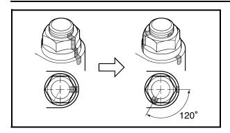
e. Tighten the nut further to reach the specified angle (120°).
