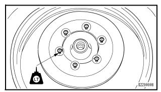
Brake disc deflection limit (maximum) Front: 0.1 mm (0.04 in) Rear: 0.15 mm (0.06 in)
