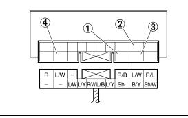
Does the starting circuit cut-off relay have continuity between black and blue/white?
