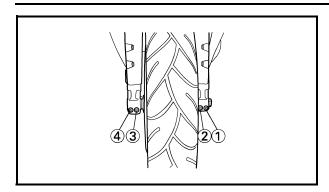
8. Tighten wheel axle pinch bolt ①, and then pinch bolt ② to the specified torque.
