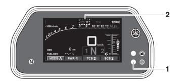
The engine operation is not normal and the engine trouble and system warning light comes on.
