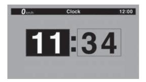
3. Set the hour by rotating and then short push the wheel switch.
