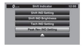
Select "IND Mode" and then select ON (to turn on the indicator) or OFF (to turn off the indicator).
