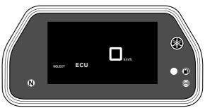
5. While "DIAG" is displayed on the display, simultaneously press the up button "1" and center button "2" for 2 seconds or more.
