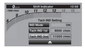
7. Set the orange color starting r/min by rotating and then short pushing the wheel switch. All r/min above this figure until the 14000 r/min red zone, will be displayed in orange.
