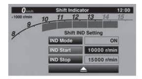
6. Select "IND Stop" then rotate the wheel switch to adjust the r/min at which the shift timing indicator will go off. "IND Stop" operational range is 8500–15000 r/min.
