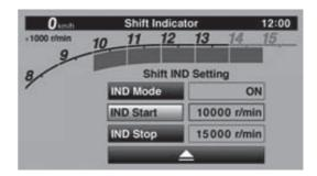
5. Rotate the wheel switch to adjust the r/min at which the shift timing indicator light will come on. "IND Start" operational range is 8000–14800 r/min.
