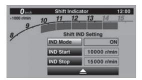
3. Select "ON" to have the indicator light steadily, "OFF" to turn the indicator off, or "Flash" to have the shift indicator flash when the indicator start threshold has been reached.
