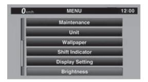
2. Select the desired brightness level by rotating the wheel switch, and then short push the wheel switch to fix the setting.
